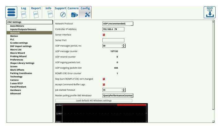
If you do know the IP address that the myCNC controller is supposed to have, confirm that it has been entered correctly. Typically, the myCNC controllers have an IP address set to 192.168.4.78 by default. Some older controller boards (usually purchased before 2017) may have a different default IP address, for instance 192.168.0.78. Enter the correct IP address and save the configuration settings. If this does not resolve the problem, go to step 2.
