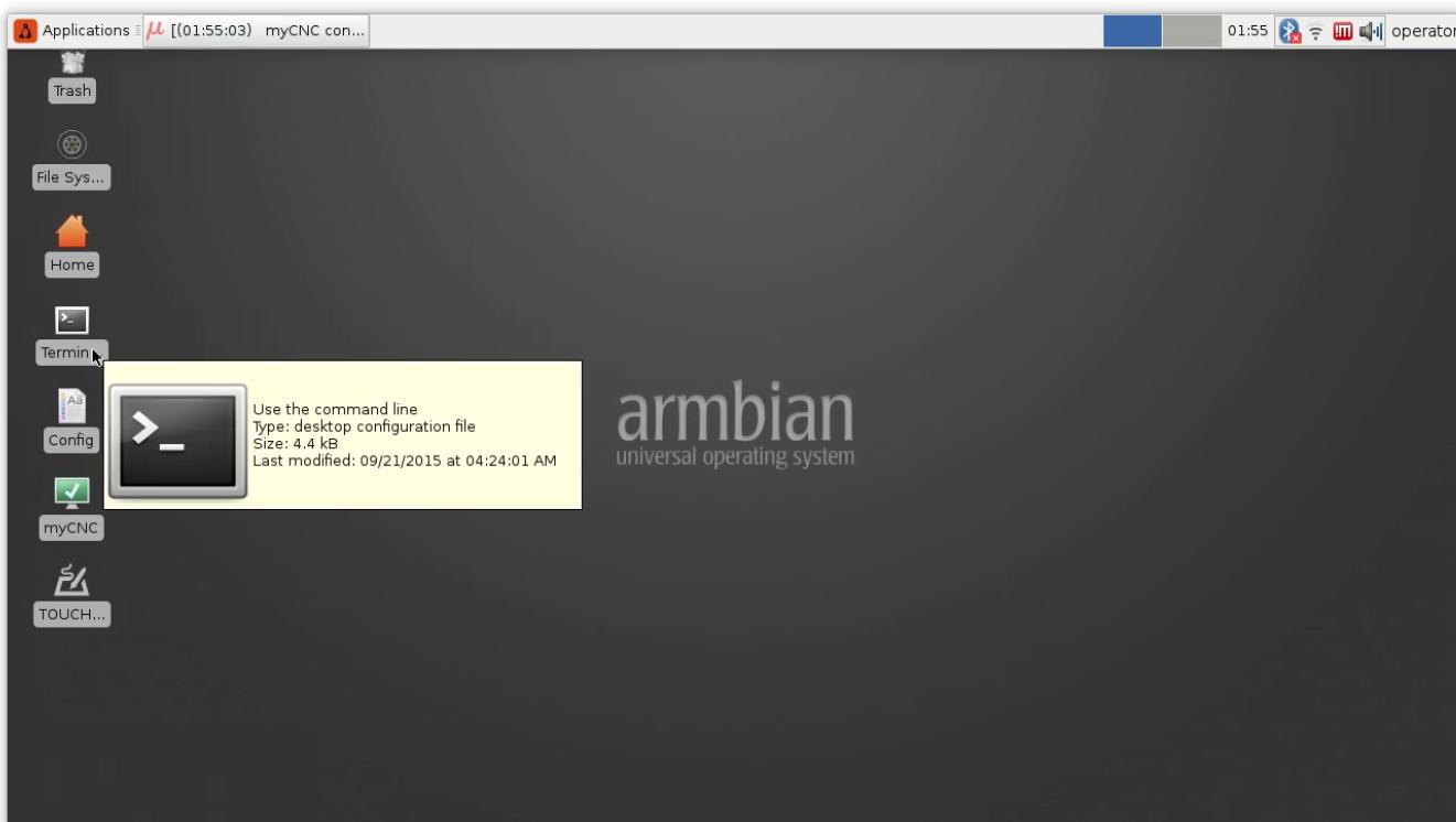
myCNC controller default IP address is usually **192.168.4.78** or **192.168.0.78**. Try to ping the board. Type command
