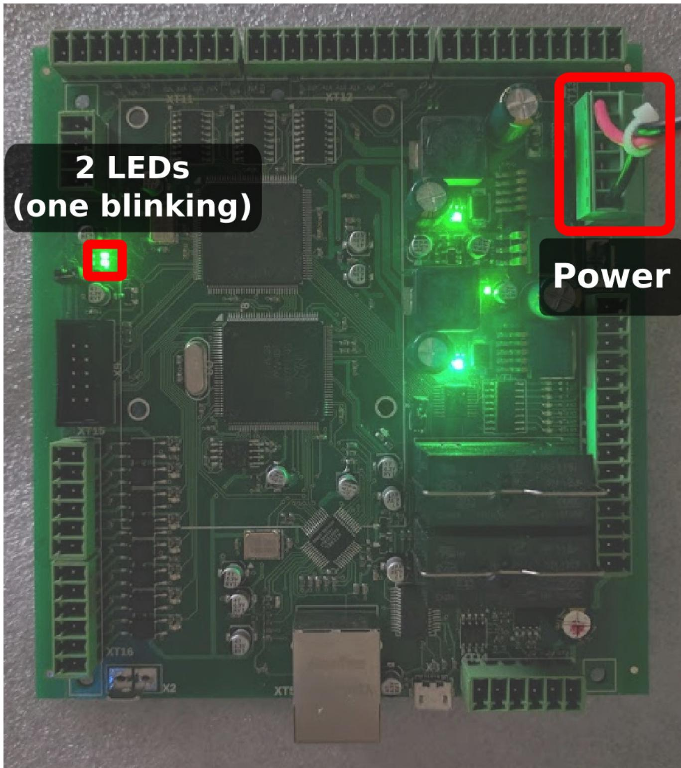
Overall, 5 LEDs should light up after supplying power to the board.
