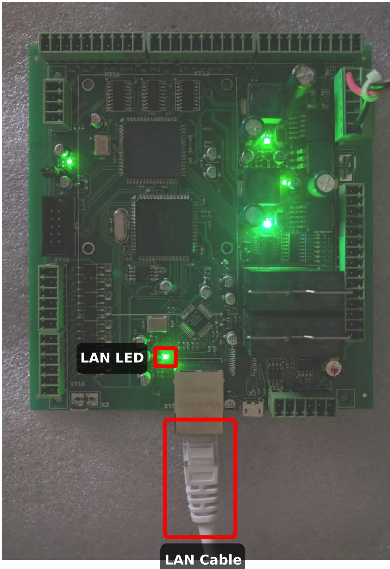
Overall, 6 LEDs (with one of them blinking) should be light up at this point.
