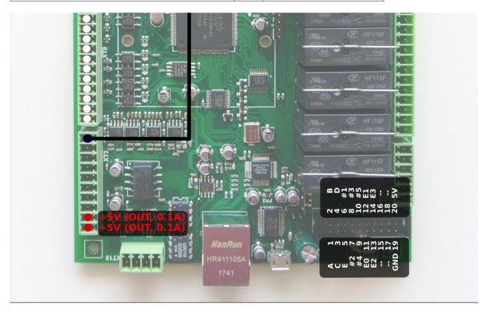
These pins are actually Binary inputs #16, #17, #18, #19 which are permanently configured as Encoder#0 and Encoder#1 in myCNC-ET7 controller firmware. This is the reason Slow Encoders #0, #1 configuration for ET7 controller in myCNC software is ignored and can be skipped. However, Encoder #2, Encoder#3 can be attached to any or binary inputs and configured accordingly when using the ET7 board.
