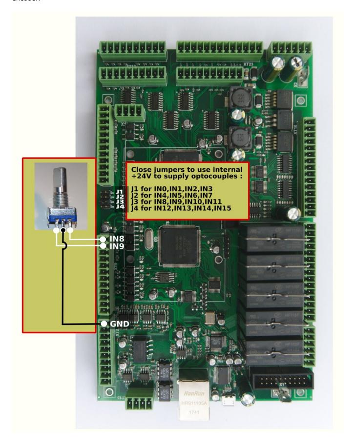
Encoder should be set up in the **Config > Inputs/Outputs/Sensors > MPG through binary inputs** configuration dialog.
