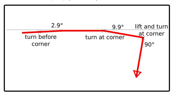
As can be seen in the example above, our Min Angle values were 3 and 10 degrees respectively. Thus, the machine will start turning the knife before reaching the 2.9 degree corner, then will continue to travel up until the 10 degree corner at which it will turn the knife again (all of that without lifting). At the 90 degree corner, however, it will lift the knife first before turning it, as the turn is too sharp for the knife to be rotated while still embedded in the cutting material.
