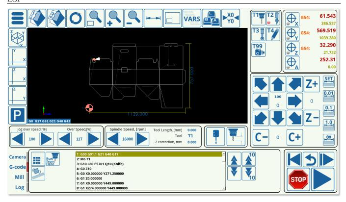
The DXF import procedure automatically generates the knife turn/knife lift G-codes which are inserted into the program, and which correspond with the settings listed in Config > Technology > Tangential Knife. This allows for easy set up provided the DXF file has been correctly modelled.
