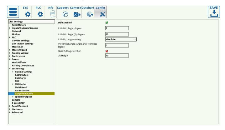
In order to enable the system, change the flag in the **Knife Enabled** line to ON (green). If you later navigate to the main screen of myCNC software, the indicator on the tangential knife icon will show whether the system is on or off, without having to go to the settings (red for ON, grey for OFF).
