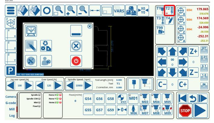
**Knife Min Angle** values signify the largest angles at which the machine will still be turning the knife without lifting it. The first Knife Min Angle value signifies the maximum angle of such a turn as to allow the machine to begin rotating the knife before reaching the corner of the turn itself. This is useful when working with pliable materials which allow for some bending, in order to achieve a cleaner overall cut.
