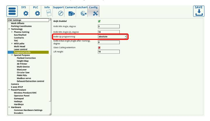
The **Angle after Homing degree** is usually left to be at zero, however that can be altered depending on the needs of the operator and the specific configuration of the machine.
