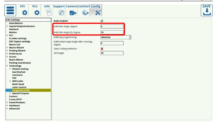
A value that is higher than Knife Min Values (meaning a sharper turn) will make the machine reach the corner and lift the knife up to its programmed lift height.
