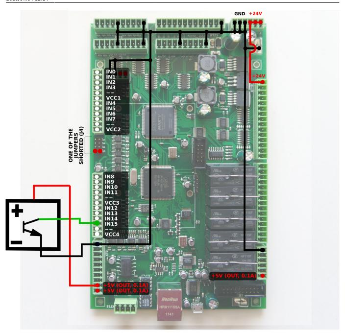
**NOTE:** The IN group of connectors used in this example is Group 4, as shown in the diagram below. Therefore, in this particular example, Jumper 4 is closed in order to supply power to Group 4. In your particular setup, please close the proper jumper for each respective group.
