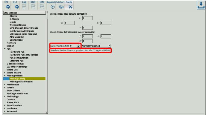
4. Double-check the TRIG04 procedure from Step 1, and edit it back to the code above if it had been changed (this can occur on older versions of the software).
