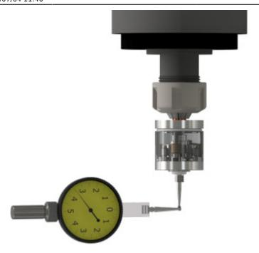
The spindle axis is moved by hand, and the amplitude of the sensor deviation is recorded using the indicator.
