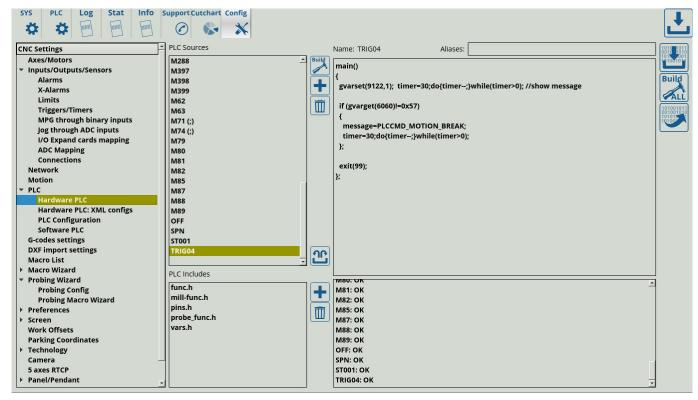
2. In CNC Settings > Probing Wizard > Probing Macro Wizard, click Generate All Probing Macros and Generate PLC Probing procedure M288. Among other settings, this generates the necessary windows for the popup screens of the probe sensor (popups 20, 21 and 22).
