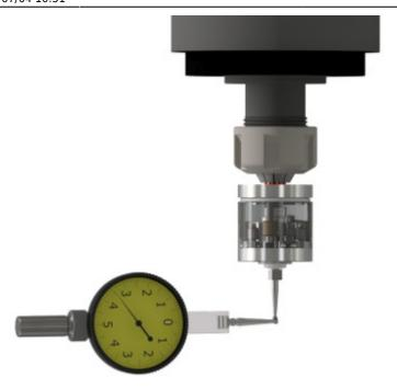
The spindle axis is moved by hand, and the amplitude of the sensor deviation is recorded using the indicator.
