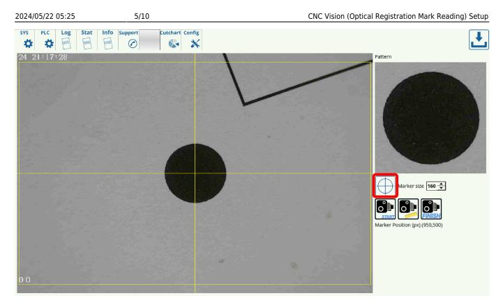
3. Press the **Start** and **Measure** buttons, and note the xy-position of the camera before moving it.
