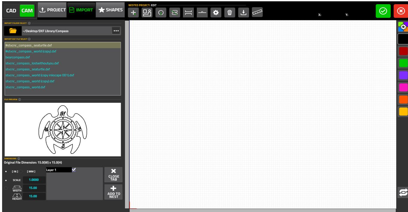
When adding a DXF file, its scale/size can be changed. This is done by selecting either the Scale or the Size of the file being imported. Below is an example of two files imported with different size/scale settings (1 and 2 for Scale=1 and Scale=2 respectively):
