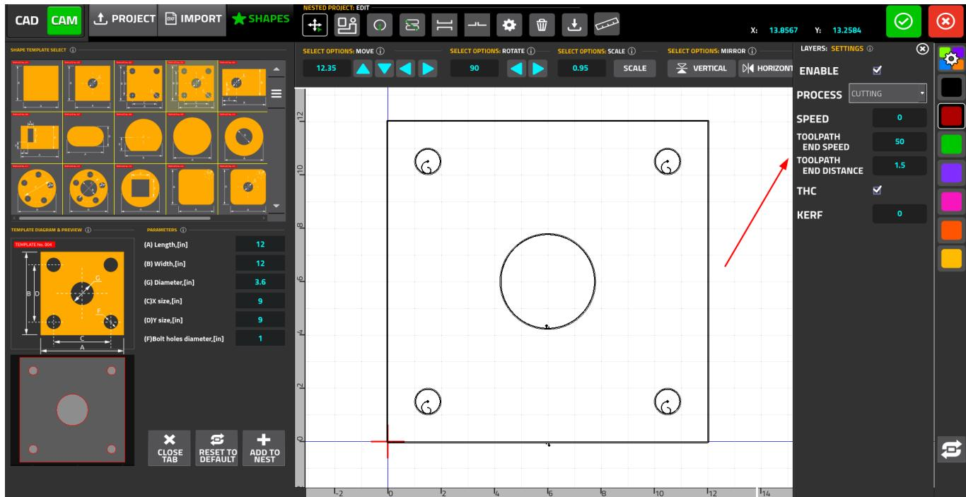
The layers are demarcated by the different colours available in the toolbar on the right. To assign a layer to a contour, select the colour (for instance, red) and click on the contour. It will change colour and will inherit the necessary settings upon import.
