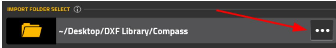
By default, the file is loaded from the folder specified in the Machine Settings (Machine Settings > Preferences > Common > NC Code Folders). However, the folder can also be changed using the Select Library button:
