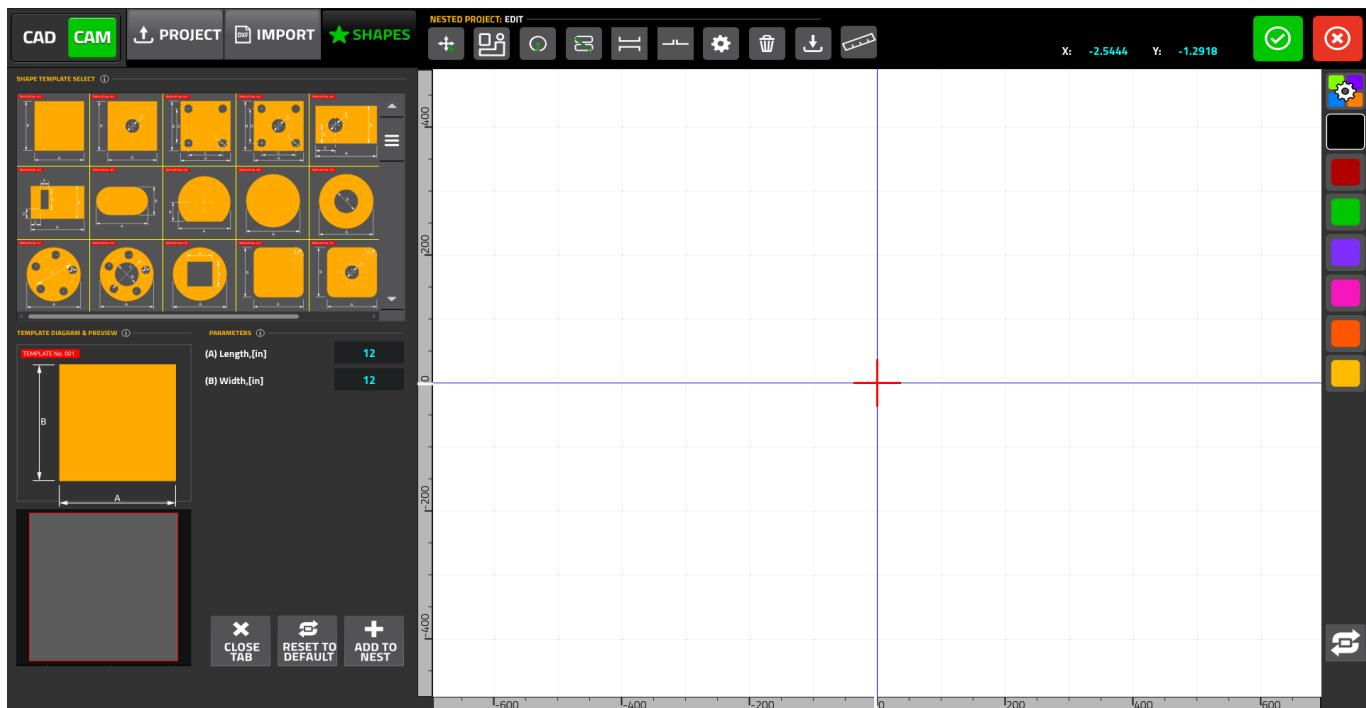
This is the list of 70+ available shapes/parts that are built into myCNC software. These include common shapes such as squares, circles, trapezoids, etc.
