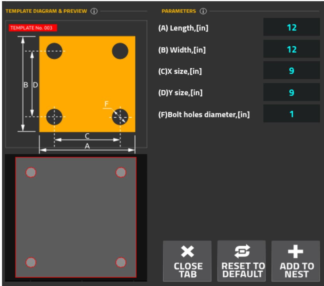
After the operator has selected the necessary custom parameters for the chosen template, it can be added to the CAM editor using the Add to Nest button. Alternatively, the user can reset the parameters of the template to their default values, or close the Shapes tab.
