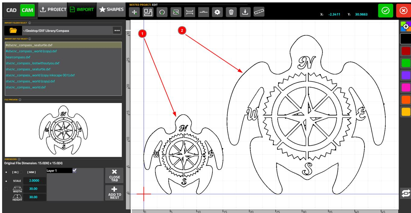
The user can also select whether the dimensions of the DXF file (which is typically unitless when created in a program such as Inkscape, etc) are to be considered to be inches or mm by default.
