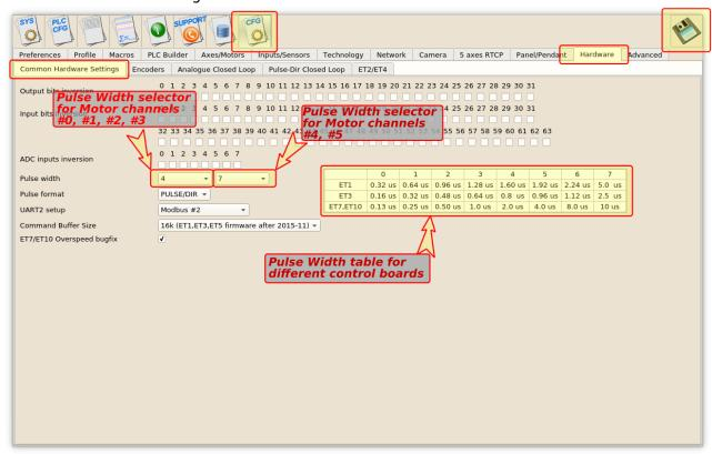
MyCNC-ET6, myCNC-ET7 controllers support separate pulse width settings for the first 4 channels (#0, #1, #2, #3) and the rest 2 (#4, #5). This option can be convenient if use high performance servo drivers with low psed stepper drivers (for example high speed servos for X, Y, Z axes and low speed stepper for rotational A axis). myCNC-ET10 controller use only the first pulse width selector for all motor outputs.
