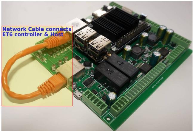
• Setup Network addresses for Host computer and myCNC Ethernet controller. Addresses of Controller and Host should be in same local network. For Example -
