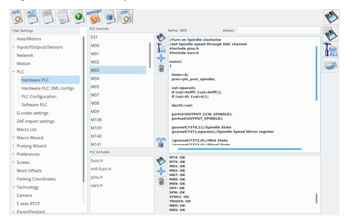
myCNC control has 2 types of built-in PLC systems that named Hardware PLC and Software PLC.
