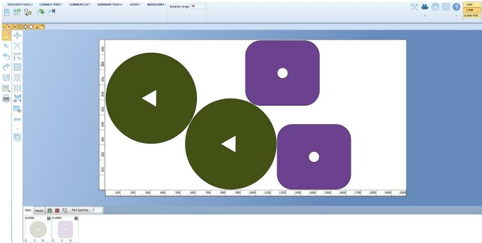
11. Click the Toolpath Tools button located in the top left corner, and then select Auto ToolPath.
