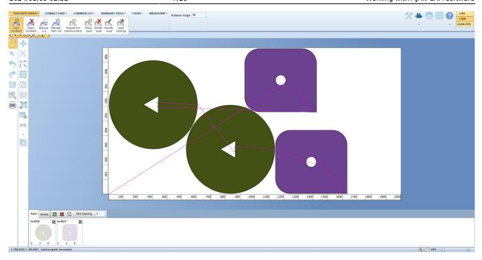
13. Once you are satisfied with how the parts and the toolpaths are set up, you can save your file as an ESSI file (.mpg).
