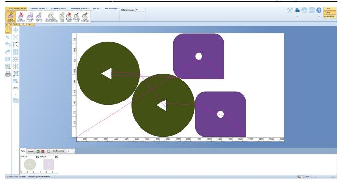
13. Once you are satisfied with how the parts and the toolpaths are set up, you can save your file as an ESSI file (.mpg).
