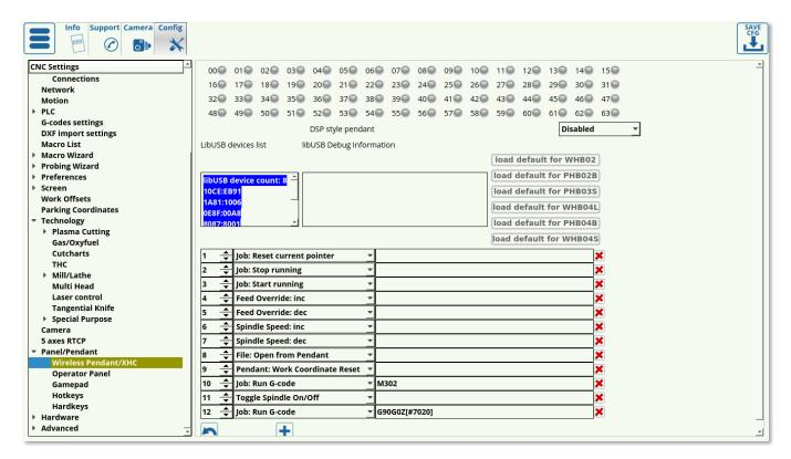
• The indicators at the top of the page serve to visually point out the pendant button which is being pressed. There indicators will light up green when the corresponding button is pressed:
