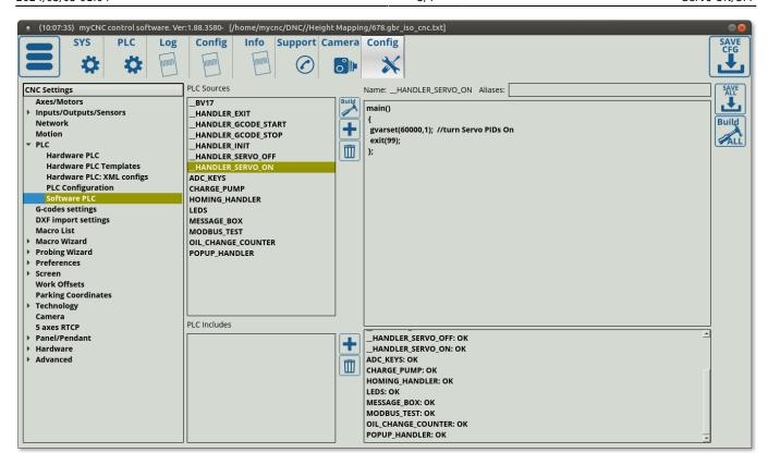
The manual code allows to use buttons to turn on and off the servo motor such as seen in the X1366P Plasma profile:
