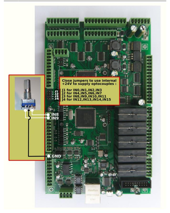
Encoder should be set up in the **Config > Inputs/Outputs/Sensors > MPG through binary inputs** configuration dialog.
