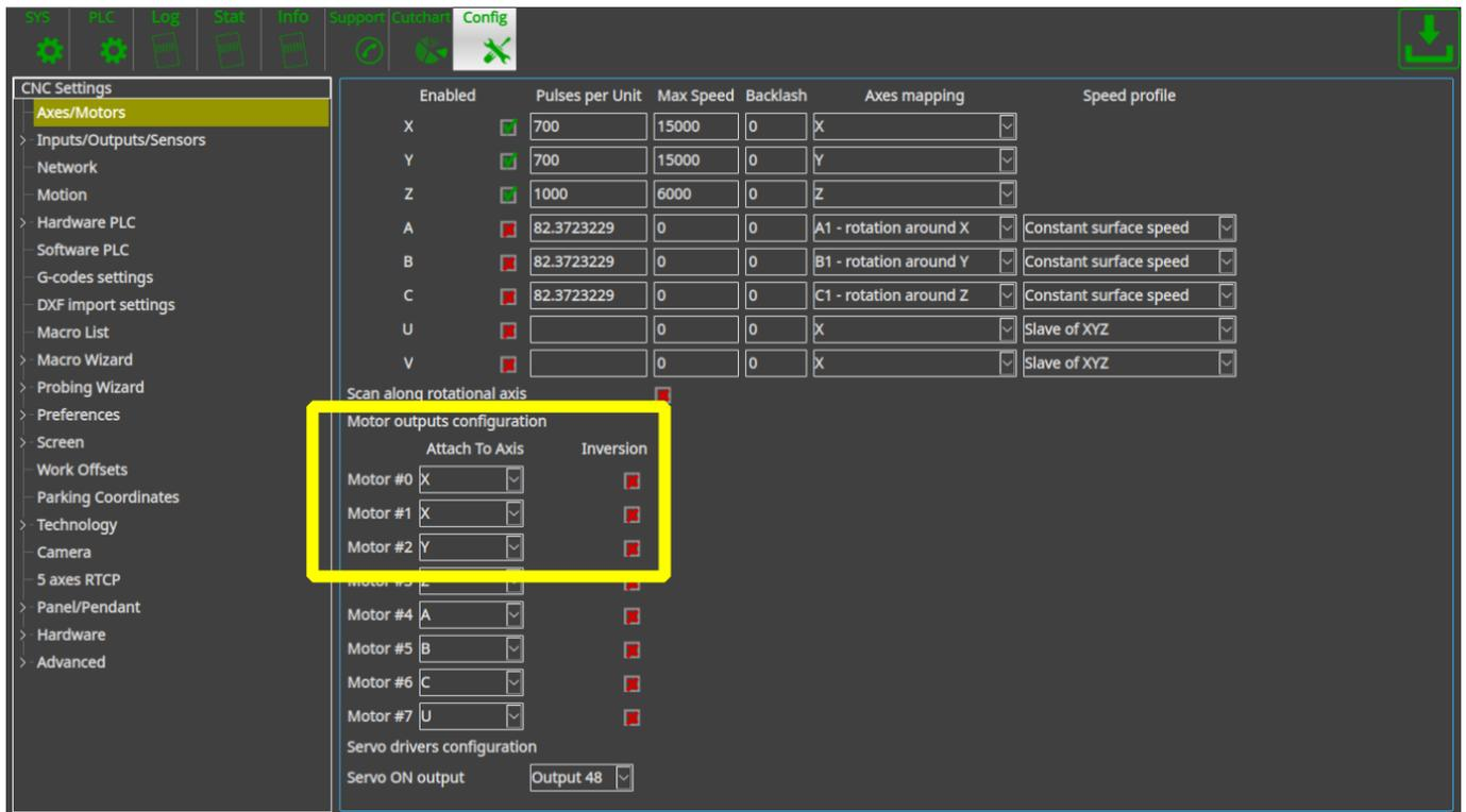
Next picture shows how to attach the Y axis to motor outputs #1, #2.
