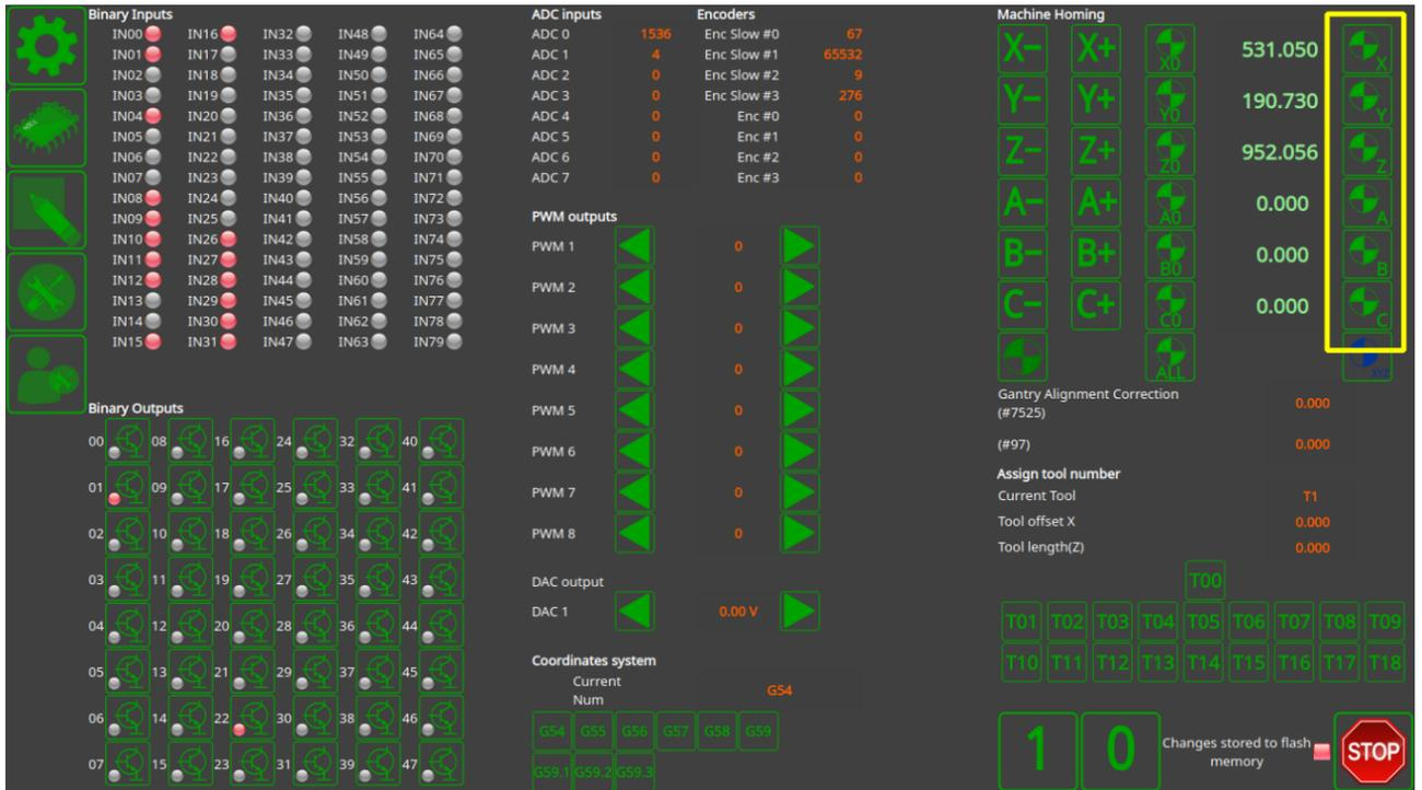
or All the Axes Homing button on the main screen of "1024P-V2" profile
