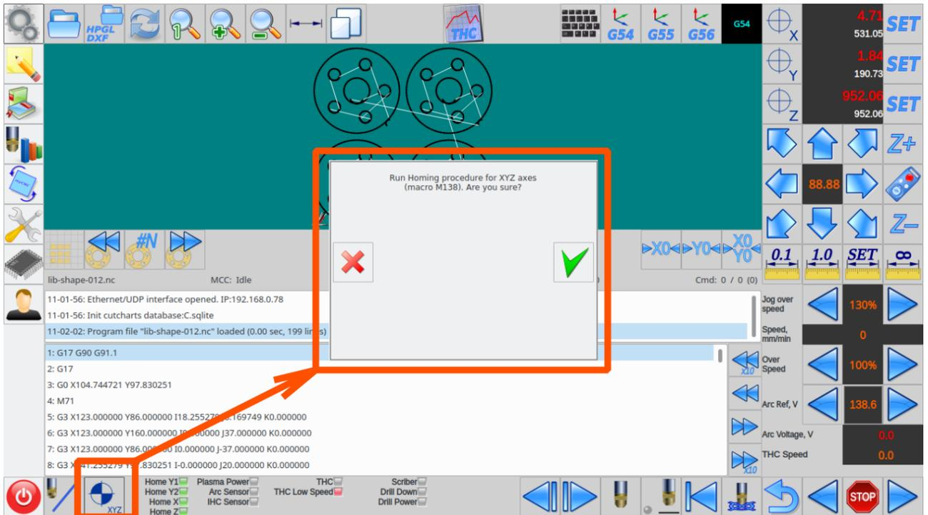
Homing Macro files should be created during machine setup. Macro file can be created
