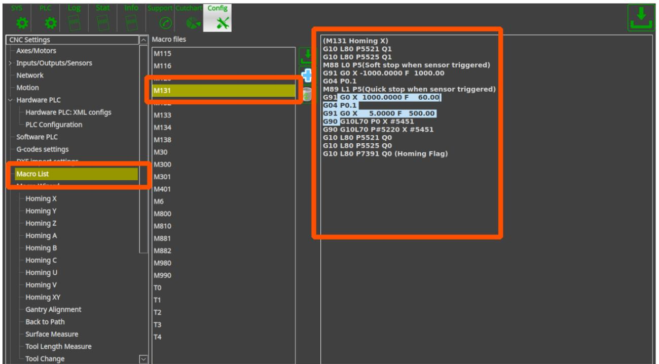
Home-All macro M138 is a simple macro file which runs in series macro files for all axes. For simple 3 axes machine it would be like this
