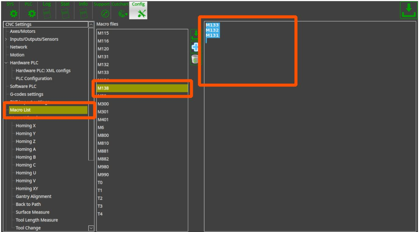
In case Gantry alignment procedure used instead of standard homing procedure, it might have different macro file name to not be mixed-up with standard homing procedure. For example - homing Y is "M132", gantry alignment is "M1321". This is just example, any of macro filename can be chosen. The result of Home-All macro would be
