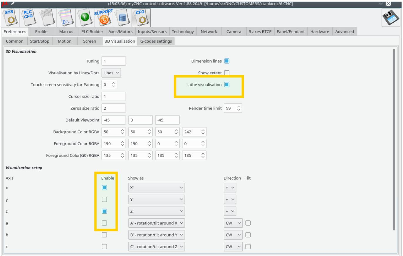
4. Check G-code settings related to Lathe operations in **Cfg - Preferences - G-codes settings** configuration dialog
