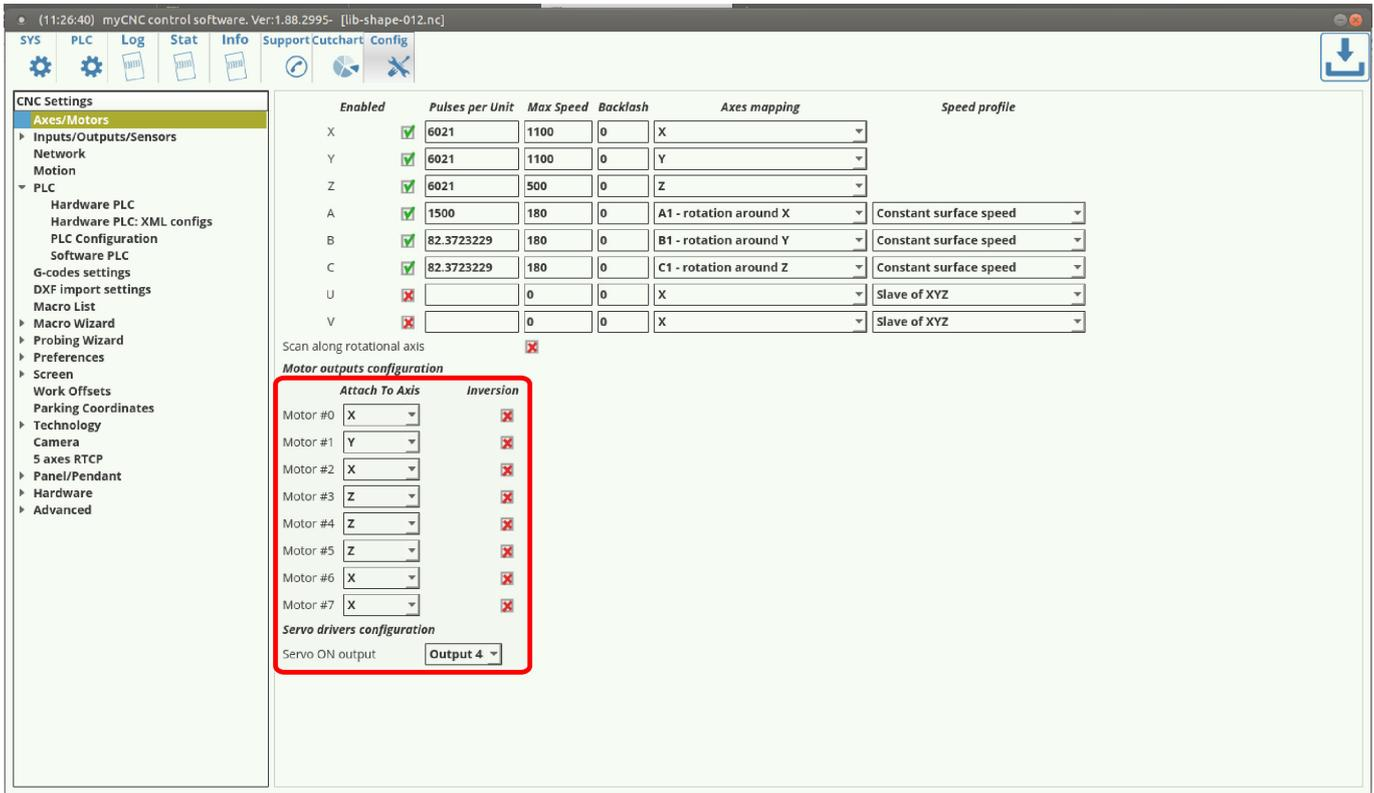
In the same window, the general calibration for the pulses per unit can be performed. This is done in order to calibrate the software readings of the machine (how much the machine “thinks” it has moved) versus the actual physical movements of the machine (how much it has actually moved). To do that:
