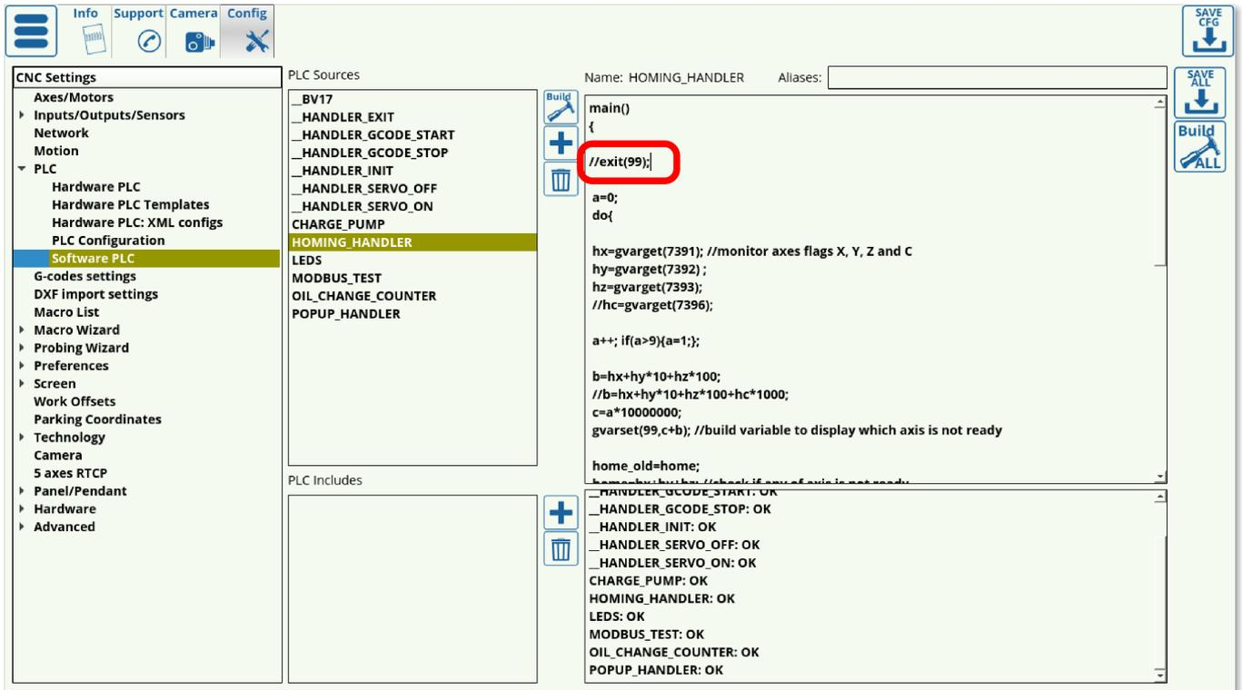
Note that the axes for which the homing is not required (Axis C in this case) have also been commented out. If only select axes need to be included in the homing procedure after the emergency stop, these can be configured in the code by adding/deleting forward slashes in front of the respective axes' commands.
