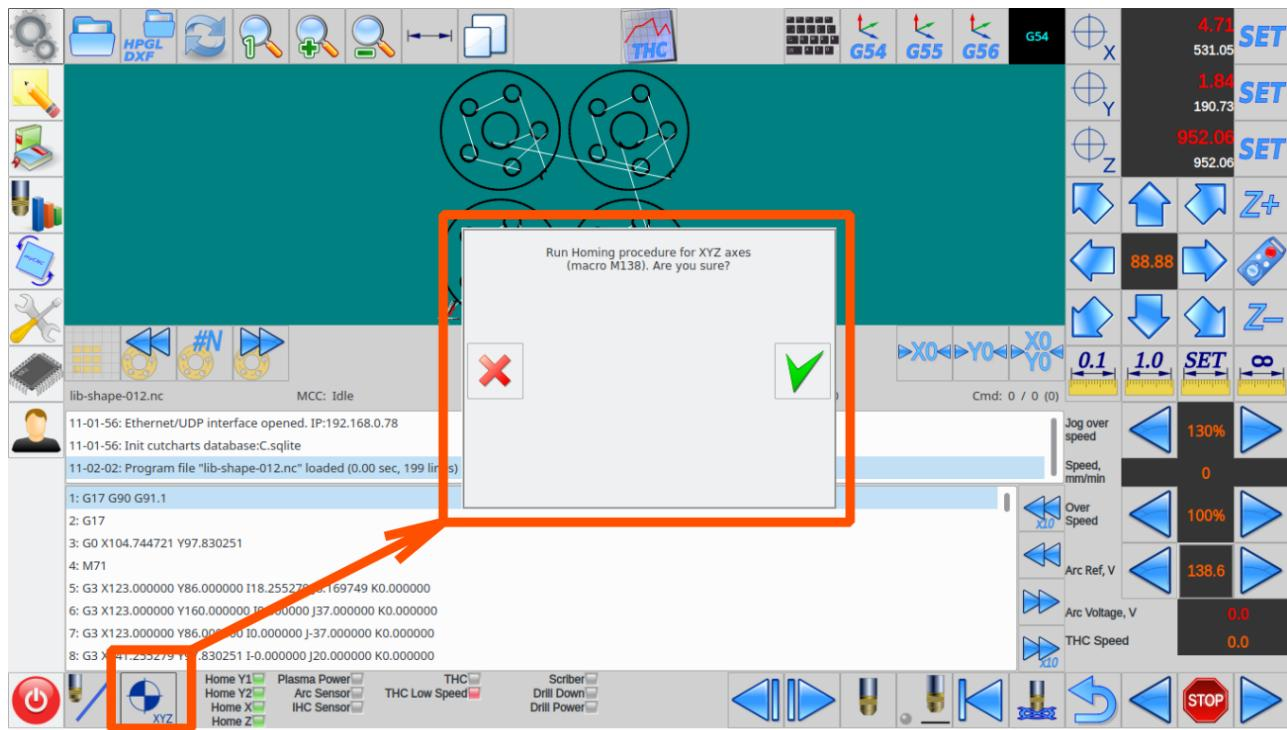
Homing Macro files should be created during machine setup. Macro file can be created
