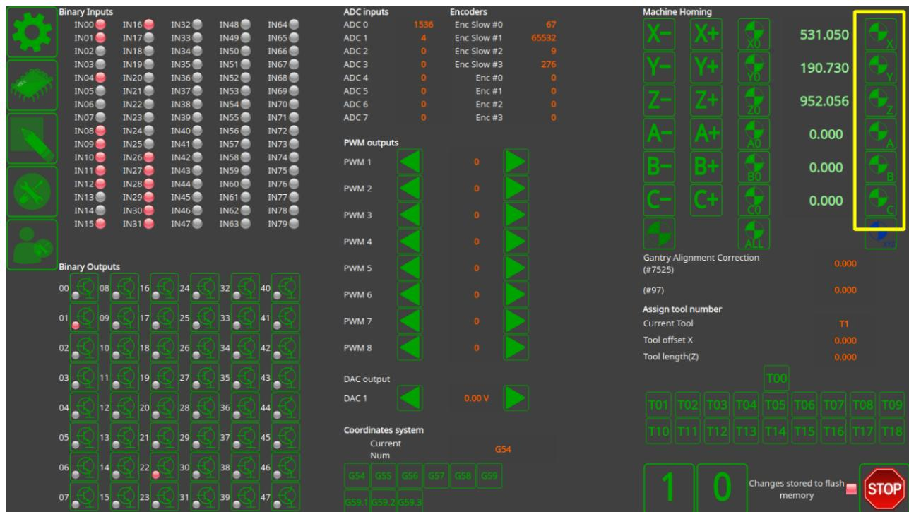
or All the Axes Homing button on the main screen of "1024P-V2" profile
