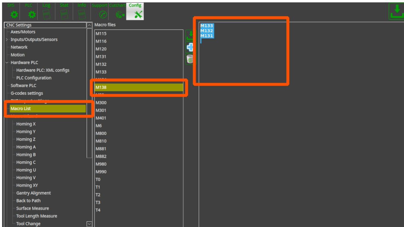
In case Gantry alignment procedure used instead of standard homing procedure, it might have different macro file name to not be mixed-up with standard homing procedure. For example - homing Y is "M132", gantry alignment is "M1321". This is just example, any of macro filename can be chosen. The result of Home-All macro would be
