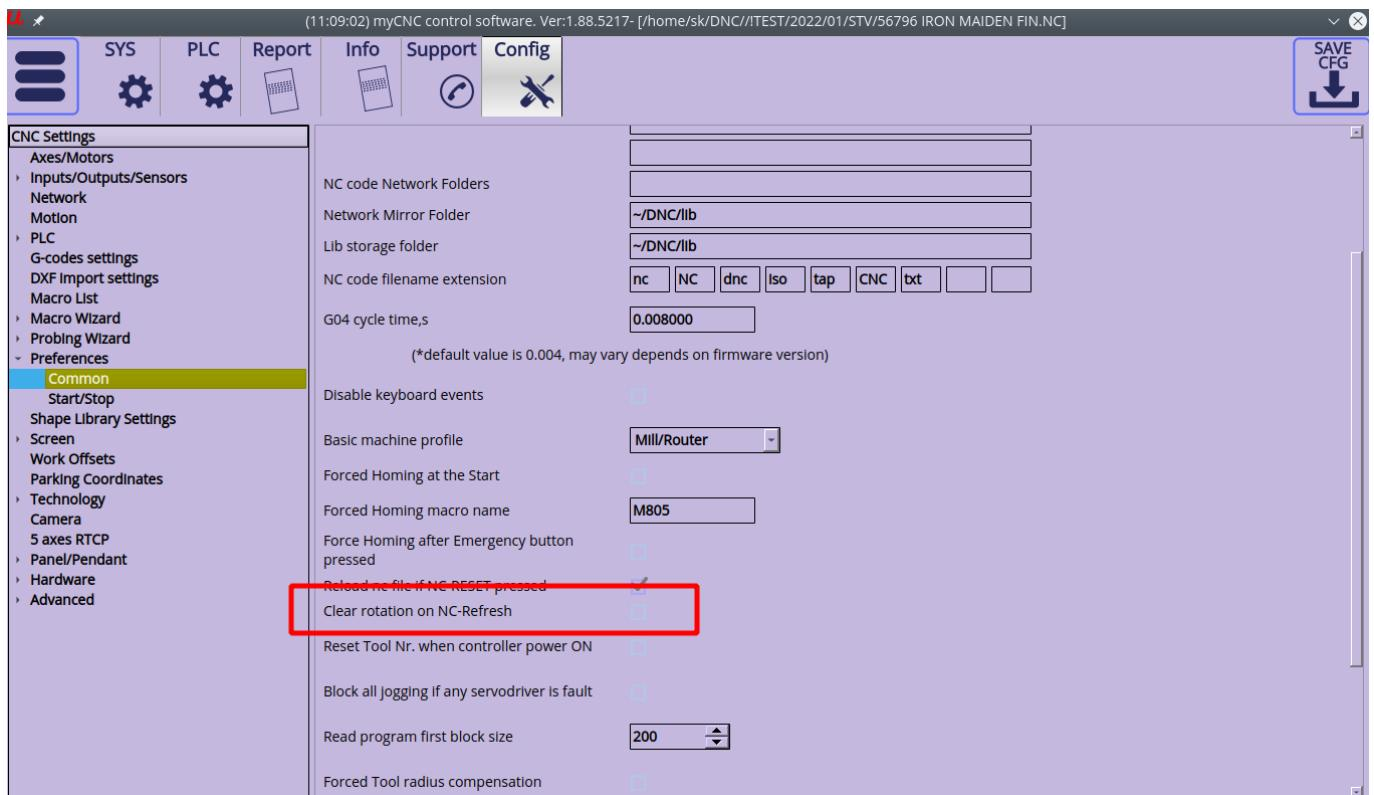
With this option enabled, the reload will now reset the rotation angle back to zero. This is useful on systems which measure the current cutting material rotation every time after loading in a new G-code file.
