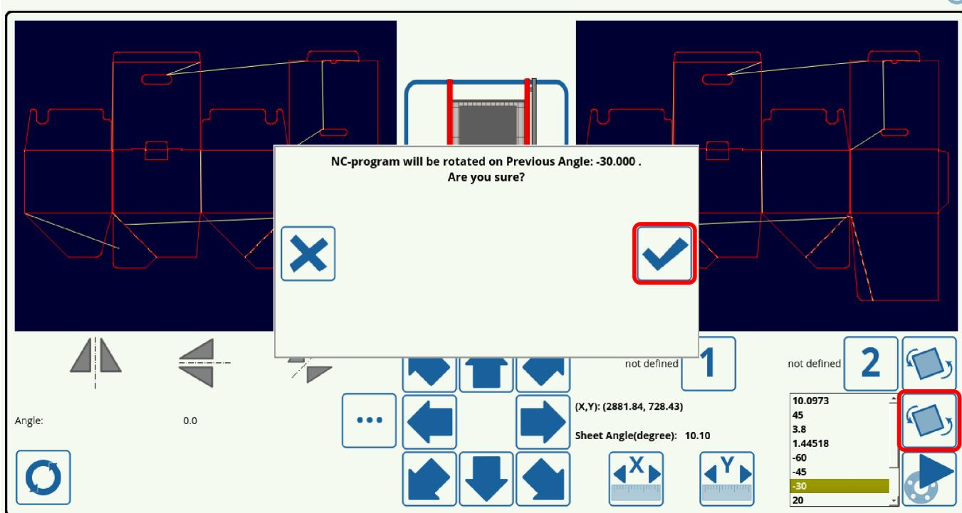
After the changes have been applied, it is necessary to press the Send button to display the rotated nesting map in the main program window so that .
