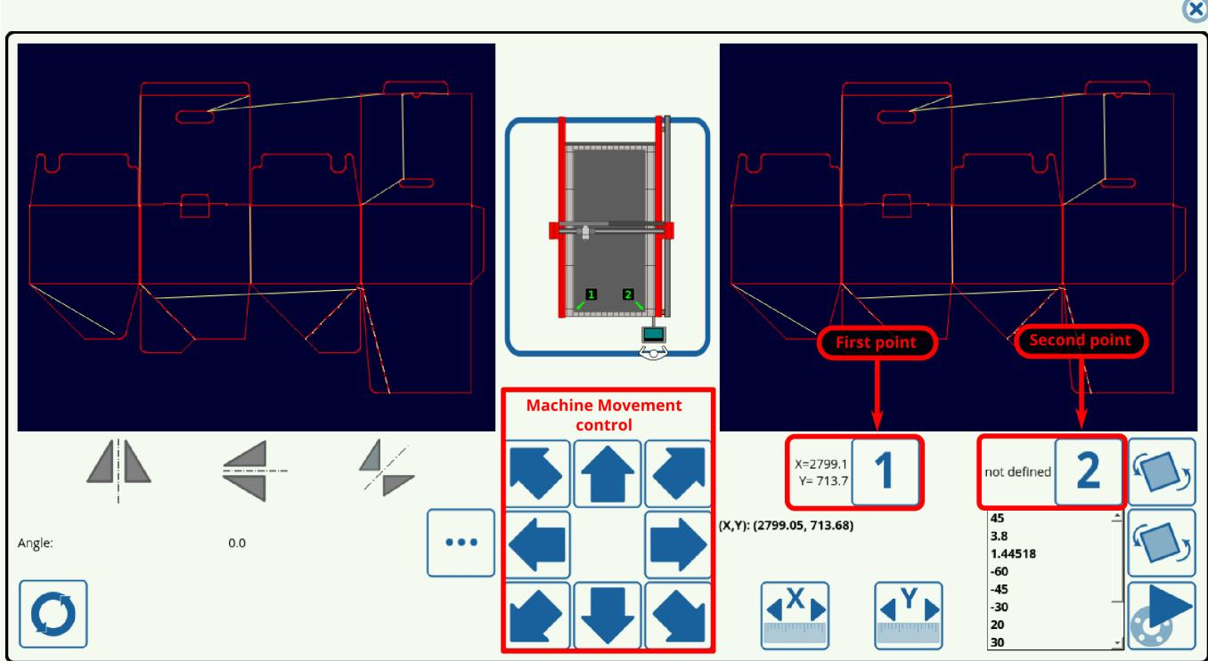
Next, move the plasma torch along the sheet (the longer the distance of this movement, the more accurate the correction will be). We bring the plasma torch to the edge of the sheet after moving along it. We assign this second point by pressing the “2” button. Movement is done with the arrows at the center of the screen.
