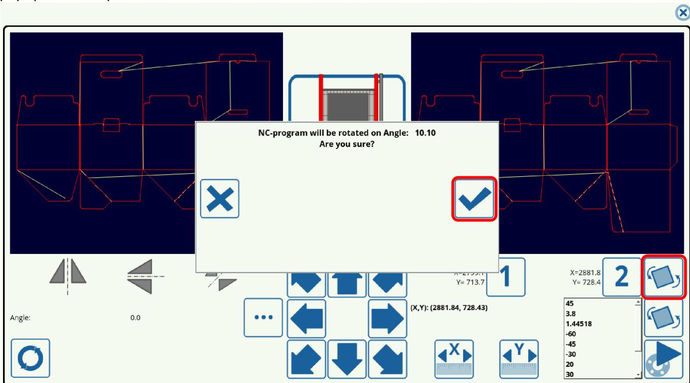
After the confirmation button has been pressed, the correction will be displayed on the screen. To use this corrected program file, it is now necessary to press the Send button to display the altered nesting map in the main program window.
