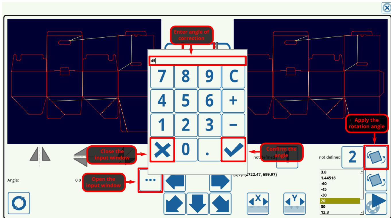
To be able to use the corrected nesting chart, it is necessary to press the Send button in order to display the rotated file in the main program window.
