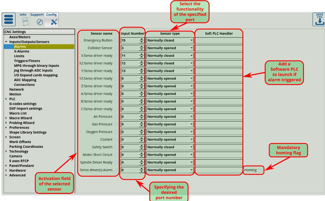
Any of myCNC controller binary input can be programmed as **Alarm** input. Alarm inputs setup is available in **Alarms** configuration dialog. In the dialog -
