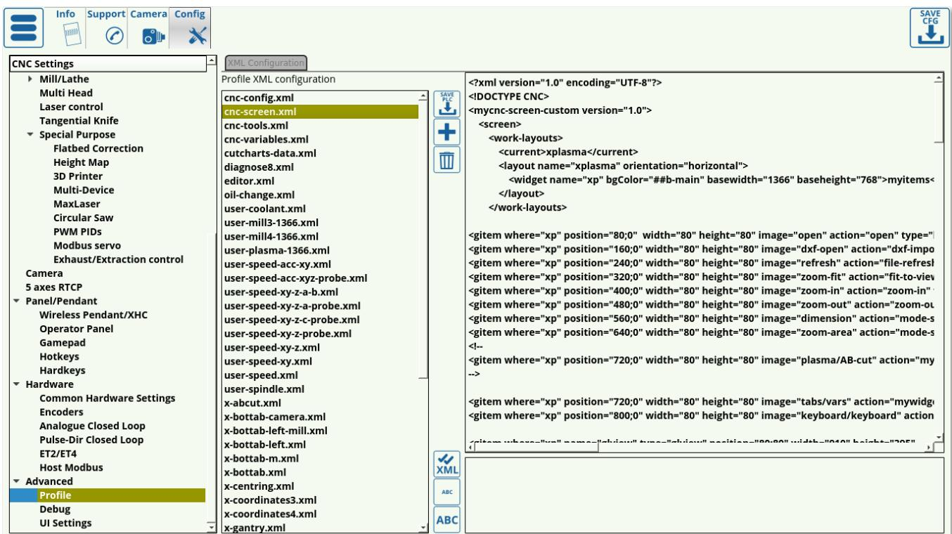
This window lists all the relevant profile xml files which define how the screen, settings, etc are laid out. These files should not be edited unless strictly necessary, as it they define the entire screen layout, the current settings config, the tools, and more.
