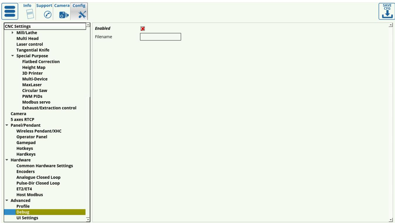
The debug window allows the user to create a debug log file. Typically not useful for end users, mostly for technical support and repair engineers.
