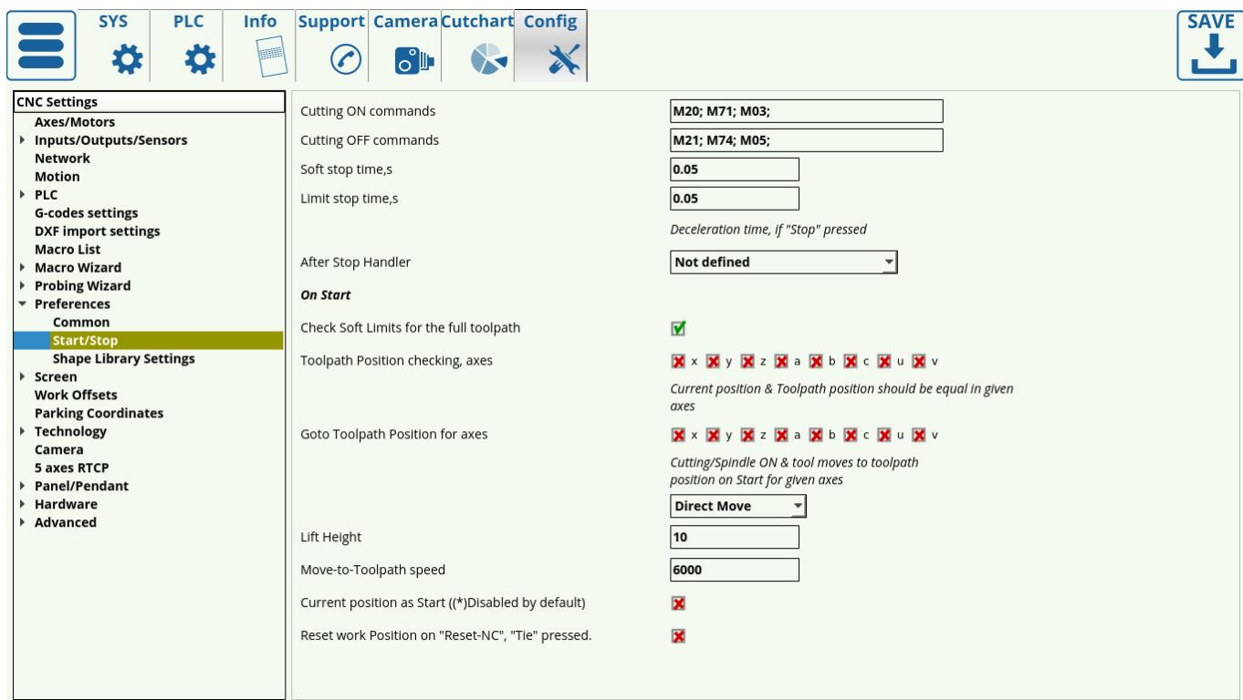
Among other settings, this window allows to edit the back-to-path behaviour on mill machines through the On Start section.
