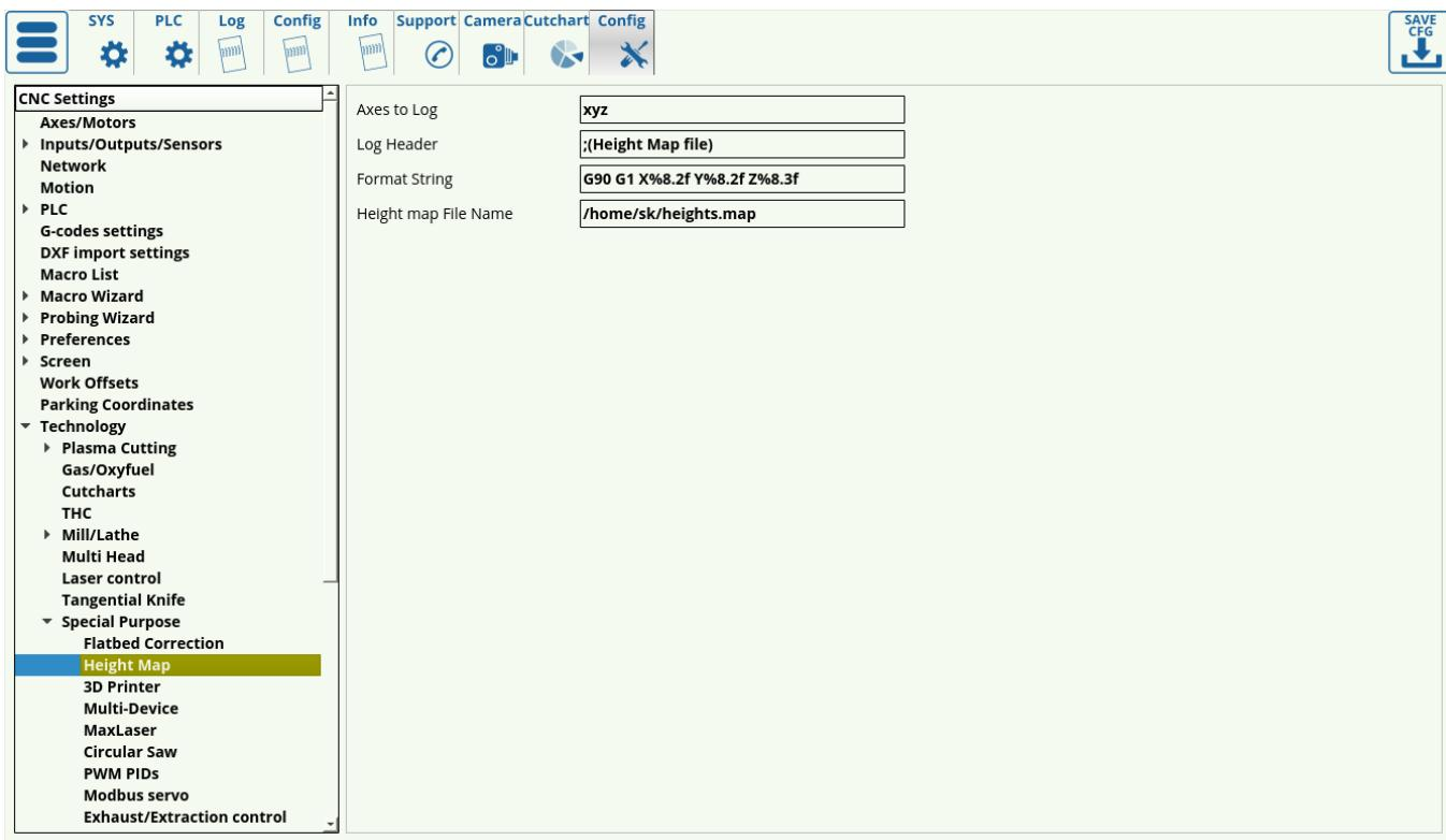
The height map is typically utilized for the per-job height probing described in the [3D Height Mapping manual](#). It is necessary to change the filepath to include the correct username for the machine (for example, /home/USERNAME/heights.map) as opposed to the default username specified in myCNC software (sk/mycnc/etc).
