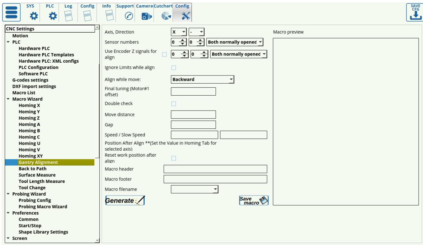
Several methods of gantry alignment can be used. By default, the method with two side sensors to move both motors will be set through this config window, however, more methods which can be set up through PLC can be found in the full [Gantry Alignment](#) manual.
