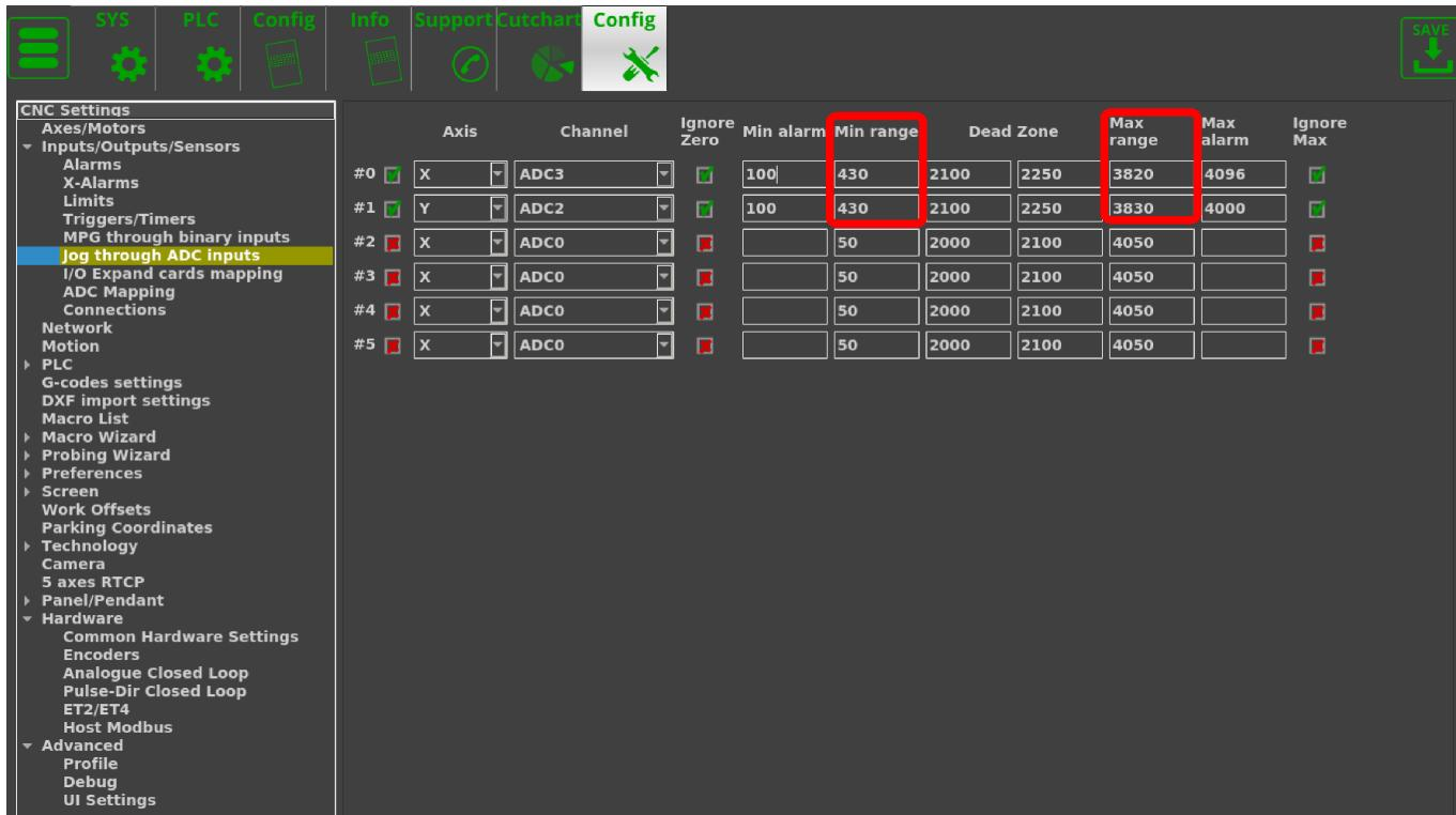
The Dead Zone is set to be from 2100 to 2150 for the joystick used in this example, as this is taken to be the zero position by letting the joystick return to its center. This value has a range so that small accidental movements of the joystick do not trigger the movement of the machine:
