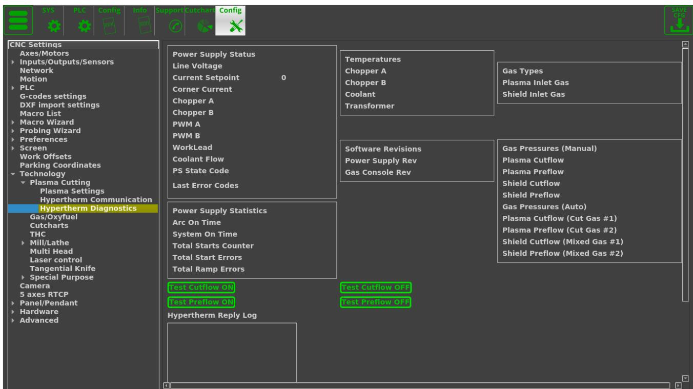
The diagnostics window is useful to see any immediate errors or problems present with the plasma machine setup, either through monitoring pressures, historical usage statistics, or temperature data.
