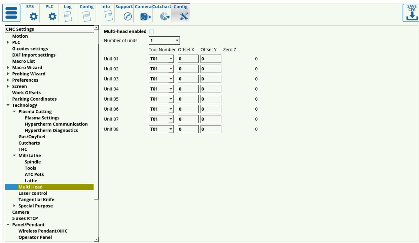
Multi Head allows for multiple tool sets. Similar to the Tools window, in that it allows for tool offsets in X and Y axes. Overall, the following settings are available:
