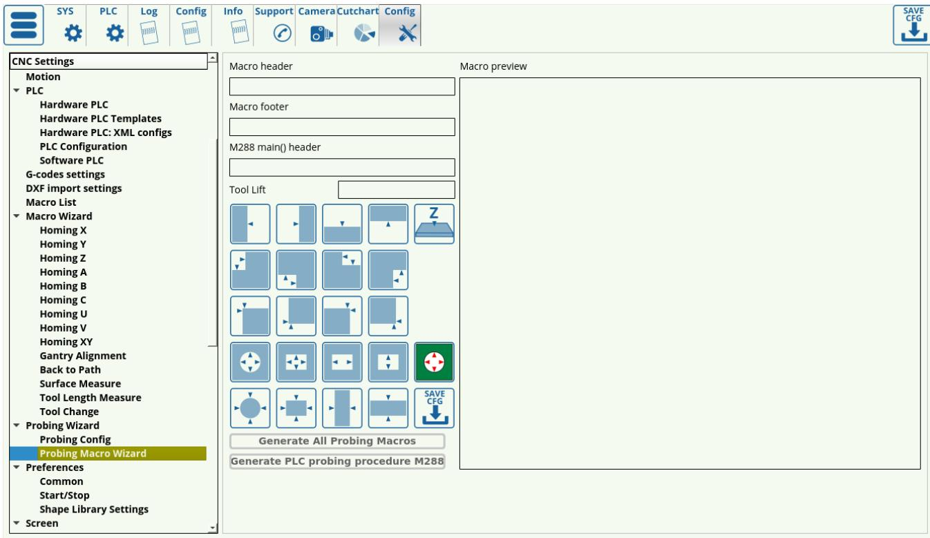
This wizard involves the macro header, the macro footer, the main() header for the automatically generated M288 macro, the necessary tool lift to safely move the probe over to the required location, and the available shapes for each of which a different macro can be generated (the macro names can be seen in the top line of each respective shape macro). These shapes allow to load in a macro preset for the particular case, and to easily edit the probing macros.
