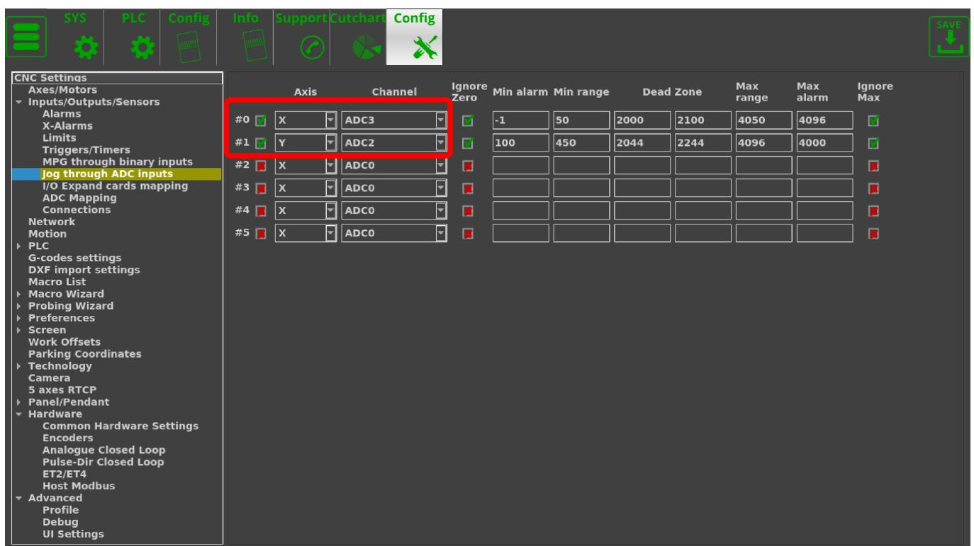
NOTE: If the axes for the joystick need to be inverted for any reason, this can be done in **Settings > Config > Hardware > Common Hardware Settings**
