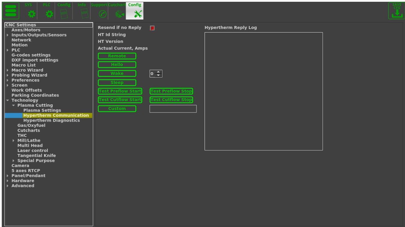
This page allows the operator to send test commands to the Hypertherm machine. The commands can be set to Remote, Hello, Wake, Sleep, Test the gas flow (preflow/cutflow channels), or a custom command.
