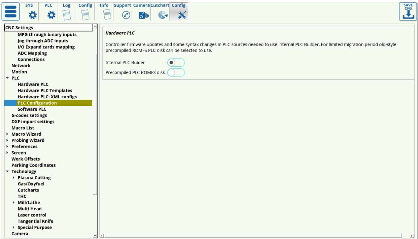
The PLC configuration window allows the user to switch to an old-style precompiled ROMFS PLC disk if necessary instead of the more recent Internal PLC Builder setup.
