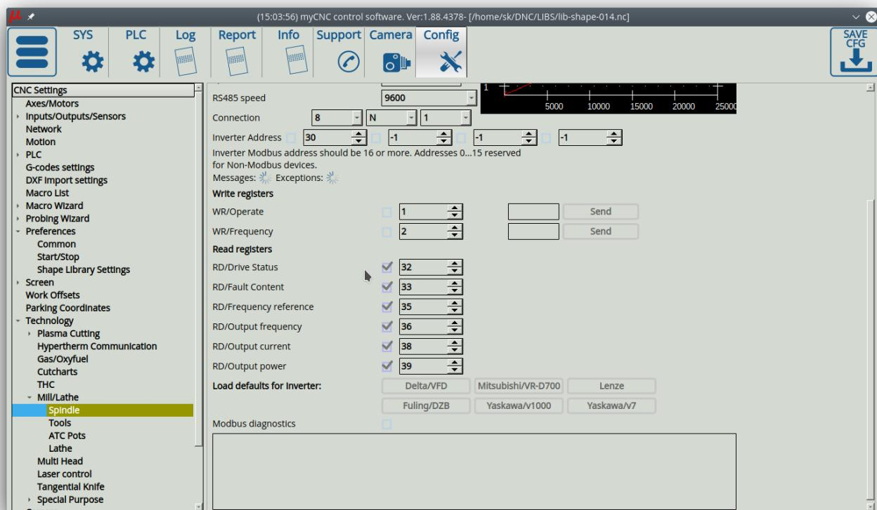
The “Read registers” values specified for read access are copied to variables # 8310 ... # 8315. The values of ordinary registers can be displayed on the screen using standard methods (LEDs, digital
