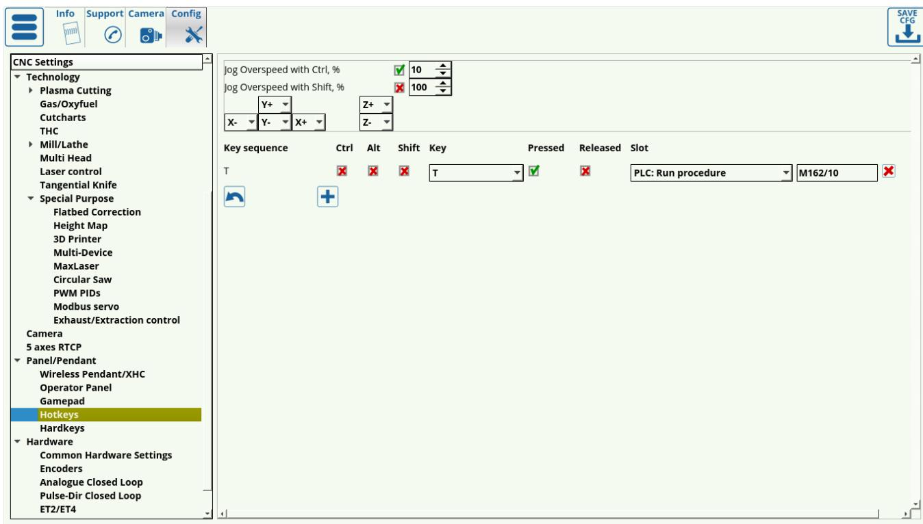
By default, the Shift and Control key are used to set different values of the Jog Overspeed %, allowing the user to quickly control jog speed with a single press. These can be set to be at different percentages (10 and 100 by default, with an allowable range of 5 to 150).
