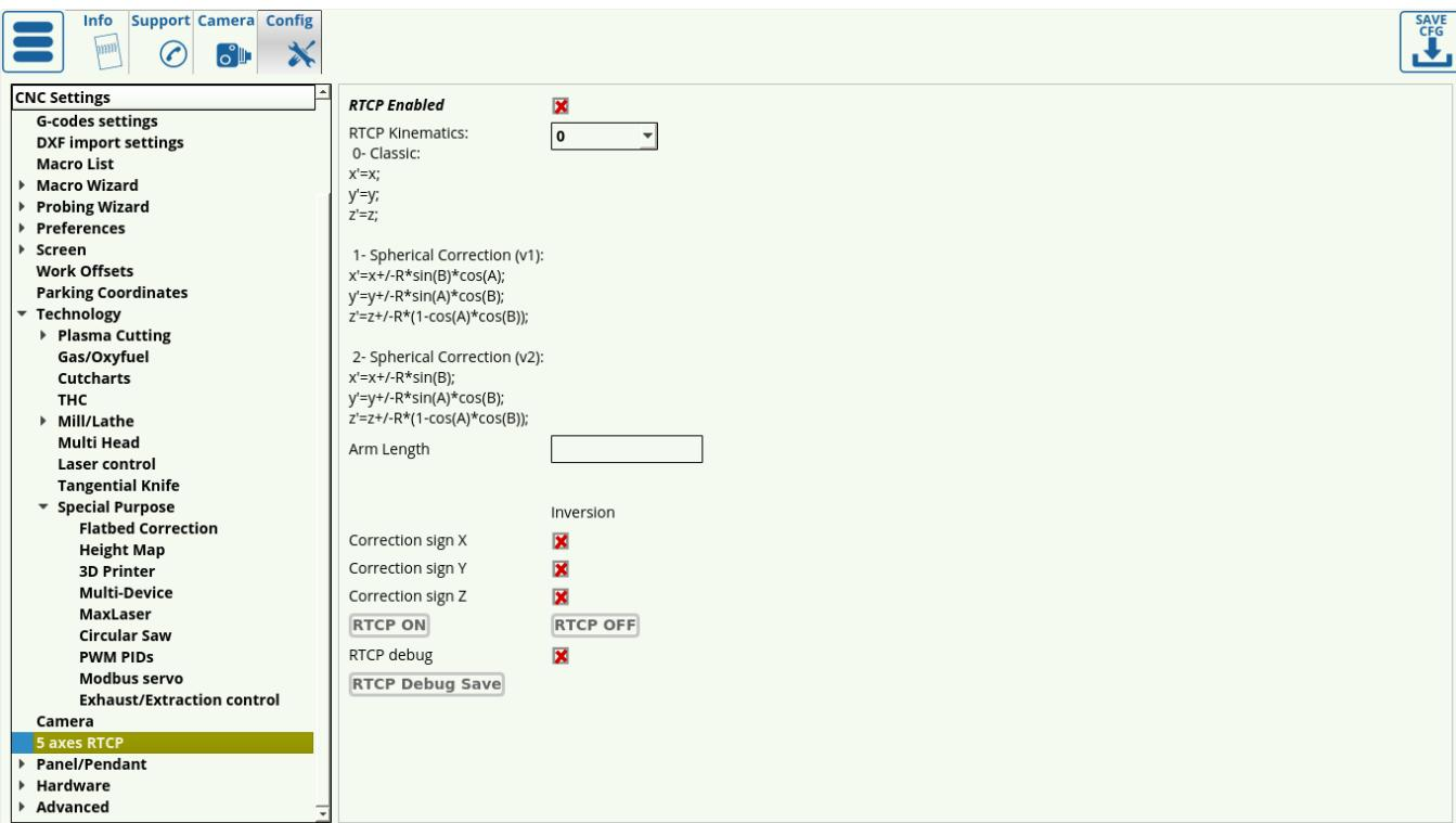
RTCP allows to compensate for a rotation of the working tool (that would otherwise lift up due to moving from a 90 degree position to a 60 degree position, for example). The following settings are available:
