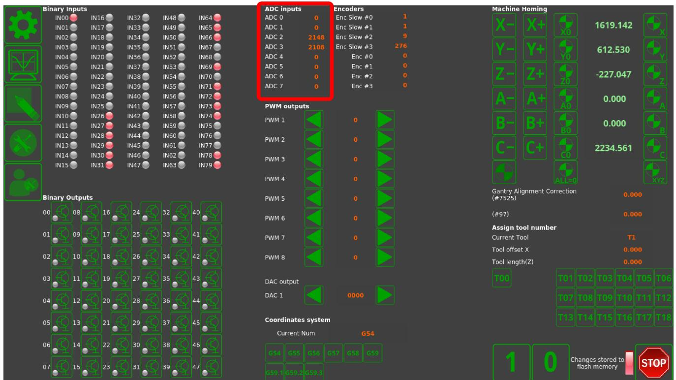
While on the system diagnostics screen, move the joystick around to check which axis corresponds to which ADC input channel. In this example, ADC2 corresponds to the y-axis, while ADC3 corresponds to the x-axis movements of the joystick. These values are inputted back on the Settings screen:
