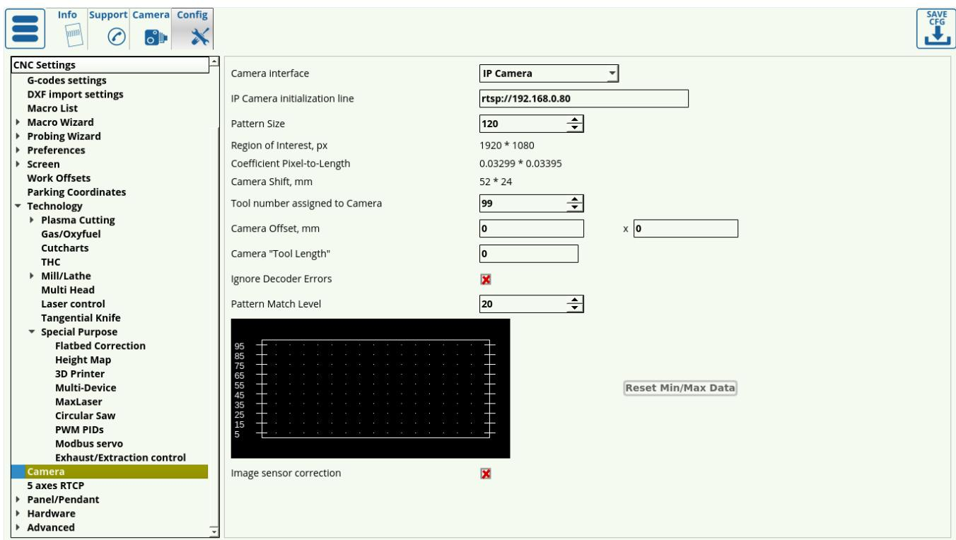
The camera system allows to correct an imported DXF file if the working material has been stretched/compressed/rotated by using reference markers (also known as registration markers, or fiducial markers) that have been calibrated using myCNC software.
