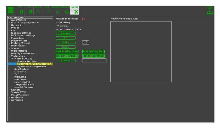
This page allows the operator to send test commands to the Hypertherm machine. The commands can be set to Remote, Hello, Wake, Sleep, Test the gas flow (preflow/cutflow channels), or a custom command.
