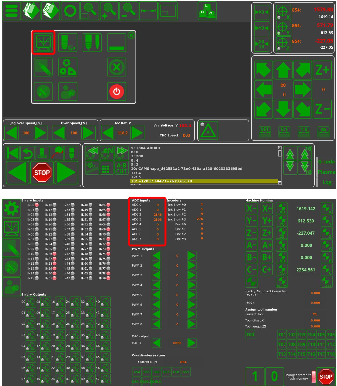
While on the system diagnostics screen, move the joystick around to check which axis corresponds to which ADC input channel. In this example, ADC2 corresponds to the y-axis, while ADC3 corresponds to the x-axis movements of the joystick. These values are inputted back on the Settings screen:
