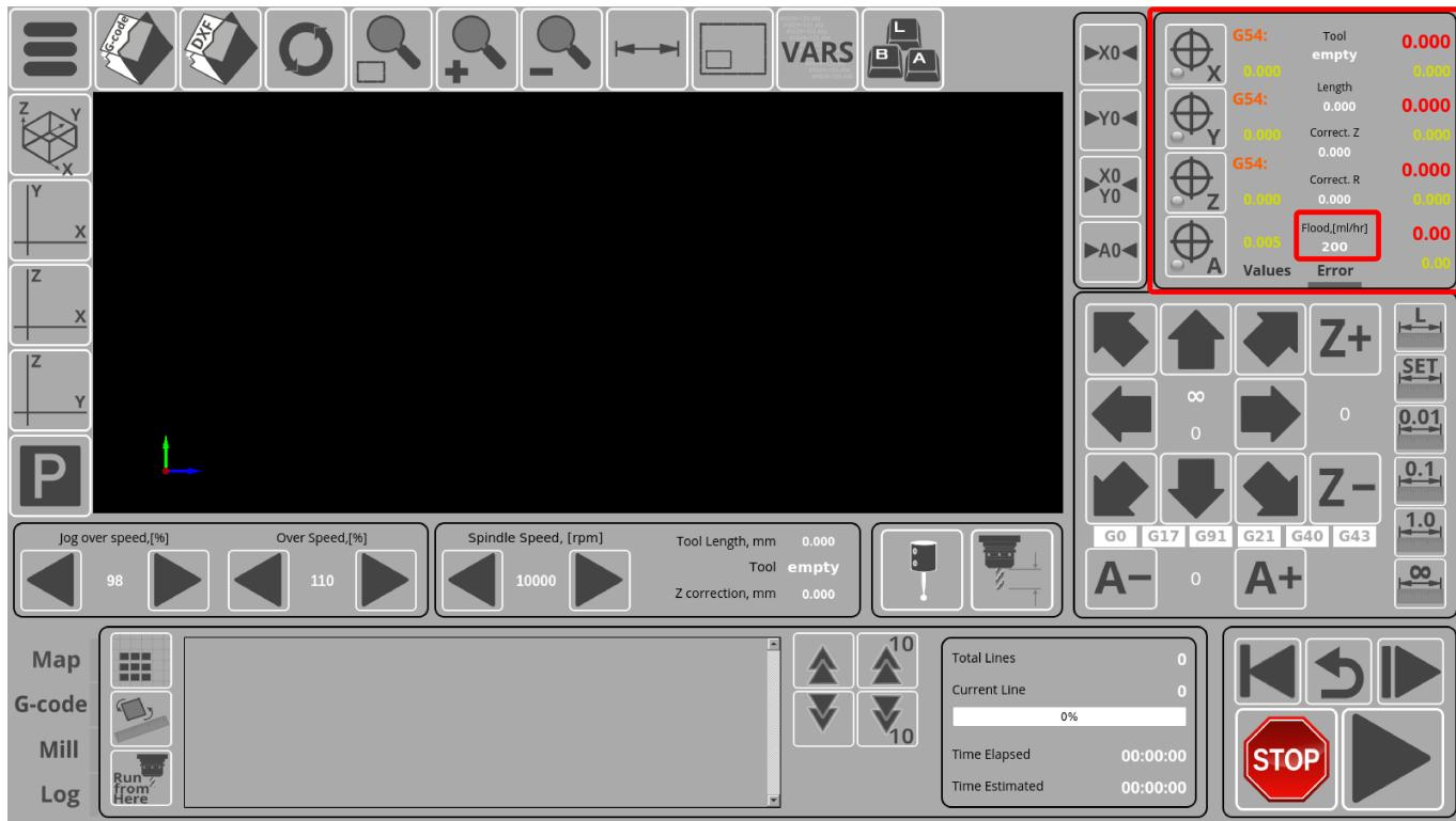
This on-screen element displays the current Flood Coolant Rate (global variable #8133).
