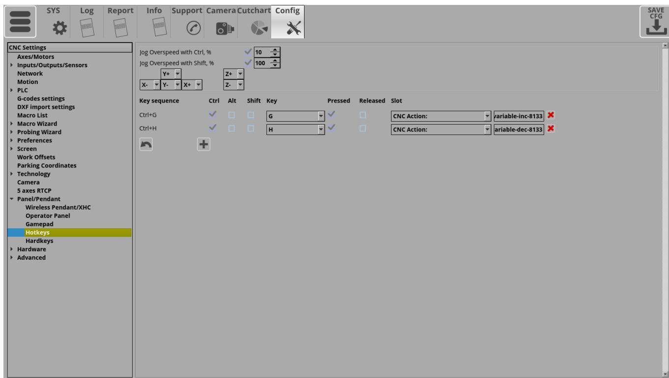
This will allow the user to quickly change the coolant flood rate from their keyboard.
