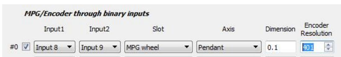
NOTE: The ET7 controller has two encoder slot reserved for the ET7 keyboard panel. These are permanently assigned to inputs #16, 17, 18, and 19, and cannot be changed despite editing the Config window (the preset cannot be overridden). If encoder input slots are to be used on the ET7 board, the latter two slots (2 and 3) should be used. This preset is not present on the ET6/ET10/ET15 boards where encoder slots 0-3 can all be used.
