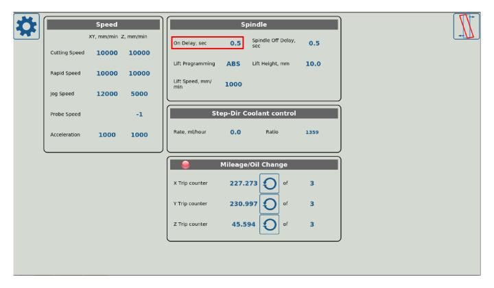
More information on controlling the spindle through Modbus can be found in the MyCNC Configuration Dialogs (Spindle) manual.
