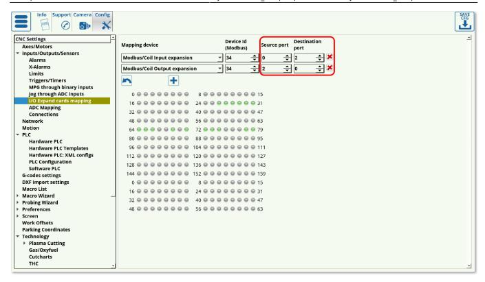
This inversion results from the Source and Destination being effectively flipped when using input/output ports via a Modbus. With inputs, the source is the Modbus device, while with Outputs, the source is the host computer/controller.
