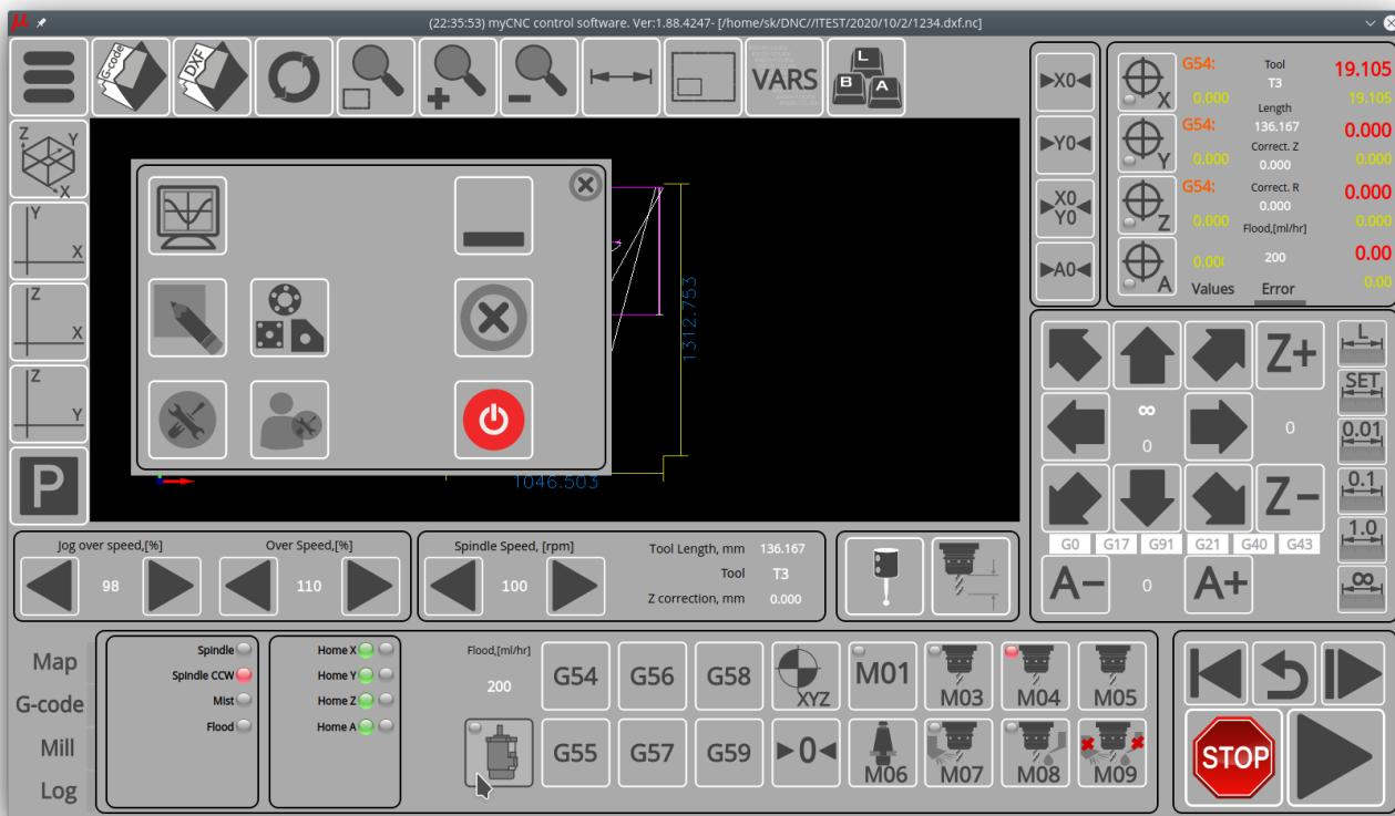
By means of a multiplier and a divider, the “software” resolution of the linear encoder must be brought to be in the “pulse-per-mm” units. In the “Linear Encoder Dimension” field, you must specify the resolution taking into account these factors and divisors, after which the controller will then operate with this program value.
