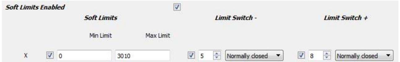
For example, the minus limit sensor is applied to the controller input 5, and the positive limit sensor is applied to the 8 input of the controller. Both shoots are normally closed.
