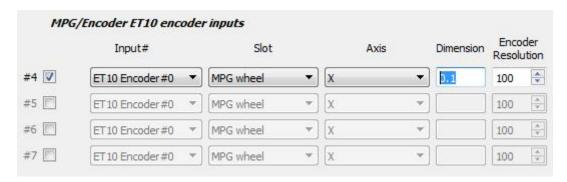
• We set the resolving power of the PGM - the number of pulses per one revolution of PGM
