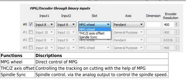
If necessary, select the coordinate axis, which will be controlled by MPG
