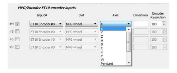
• Next we select the length of displacements with the help of MPG. Number of movements in mm per pulse MPG:
