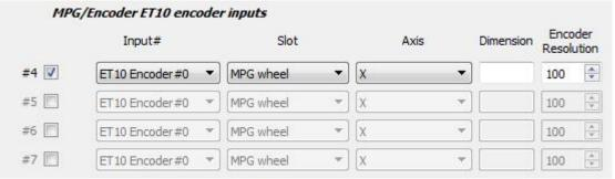
• After activation, you can select the encoder number on the controller for operating
