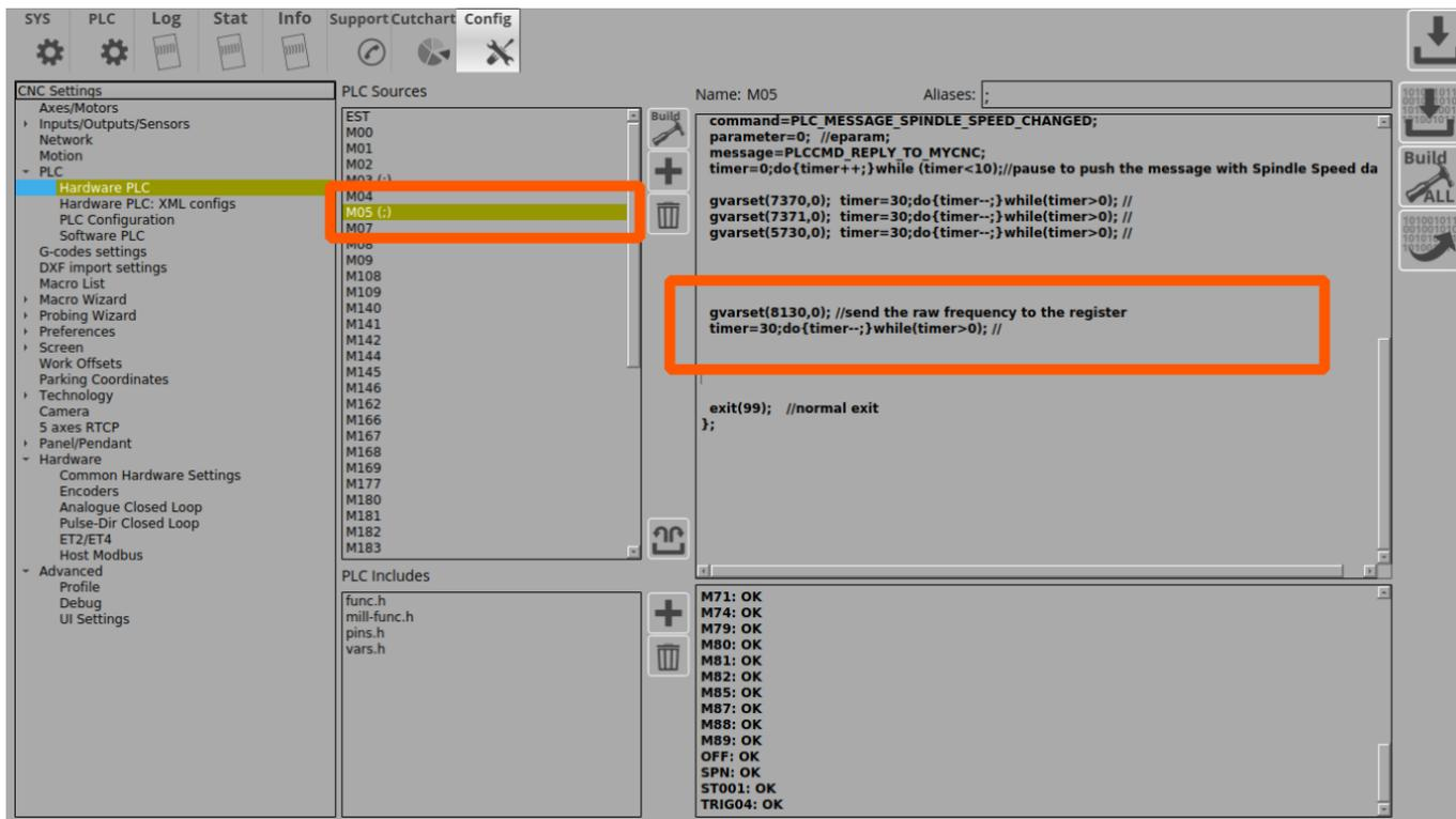
In this implementation, the pulse-dir generation will be switched ON simultaneously with the classic control (a + 0-10V relay analog output). It is assumed that an unused spindle will be shut off physically by the operator and that the additional control signal will not affect operation.
