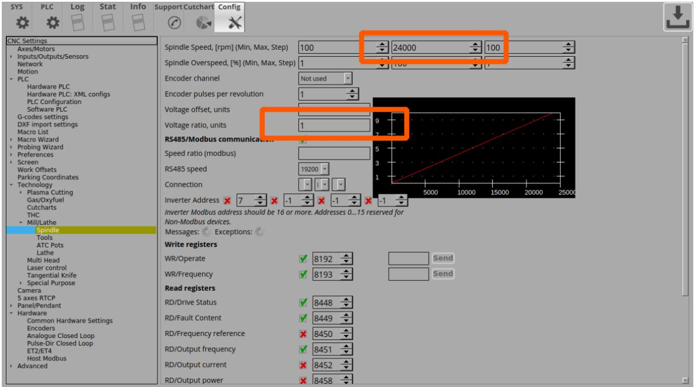
At this spindle speed, a full 10V signal must be sent to the analog output, so the “voltage ratio” coefficient is set to “1” (in the case of, for example, a spindle with an input signal range of 0-5V, this coefficient would be 0.5 to get a 5V signal at maximum speed).
