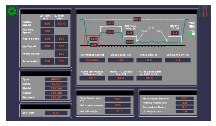
If, for example, a pneumatic probe system has been used, the IHC Ignition Height is equal to 6.0, and the IHC Correction Height is equal to 1.0, the system will go up by 7.0 mm after contact with the working surface has been made. It will then wait at this ignition height until it receives the Arc Sensor input, and will then proceed with the pierce and the THC sequence.
