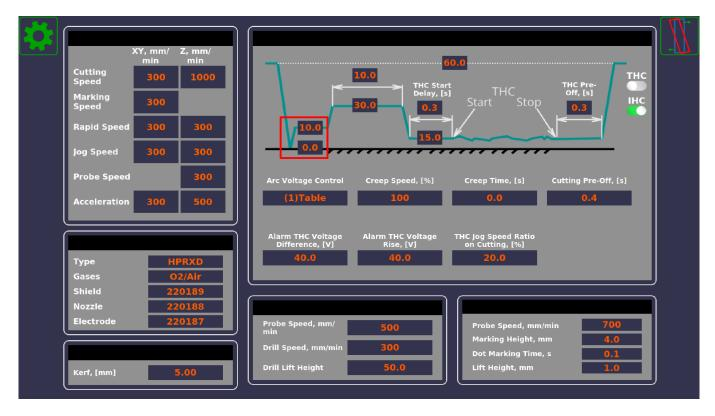
If, for example, a pneumatic probe system has been used, the IHC Ignition Height is equal to 6.0, and the IHC Correction Height is equal to 1.0, the system will go up by 7.0 mm after contact with the working surface has been made.
