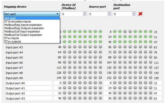
• After selecting the register for the mapping, the input or output register of the controller, where the selected registers will be redirected. An example is presented reassignment of the register of encoder inputs of the controller ET10 as a register of the controller's common inputs port 3
