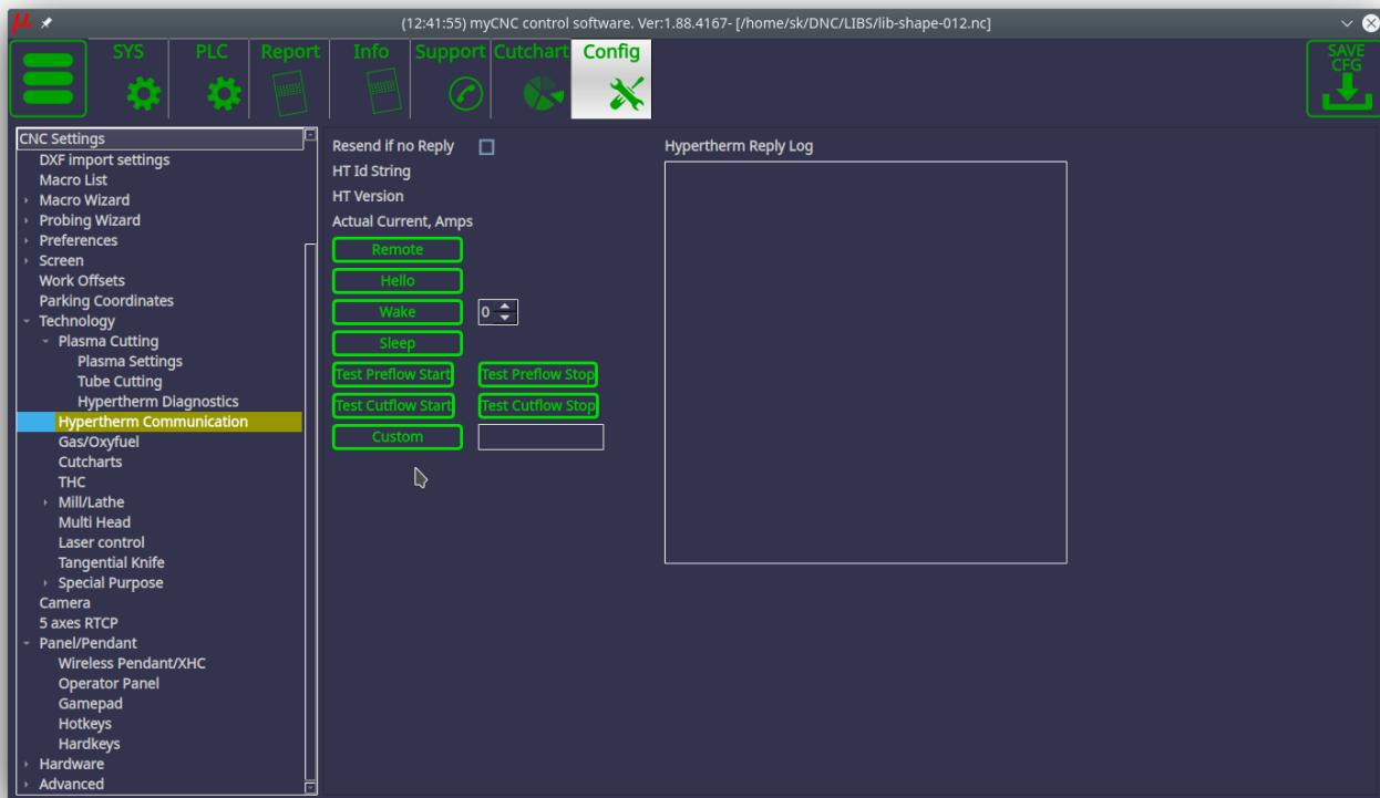
In addition, you can manually send commands for test switching on and off gases using the following buttons in the Hypertherm Diagnostics tab:
