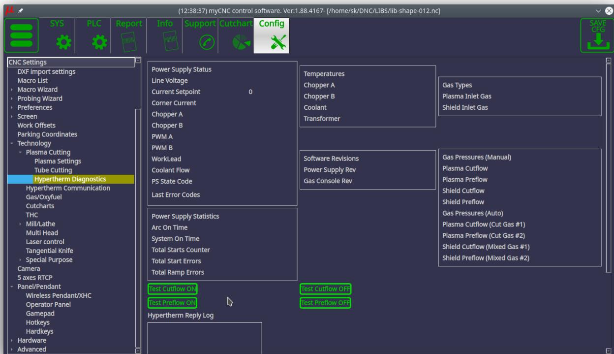
Other test commands can be sent using buttons from the Hypertherm Communication window, with the responses from the power source being printed in the Log window:
