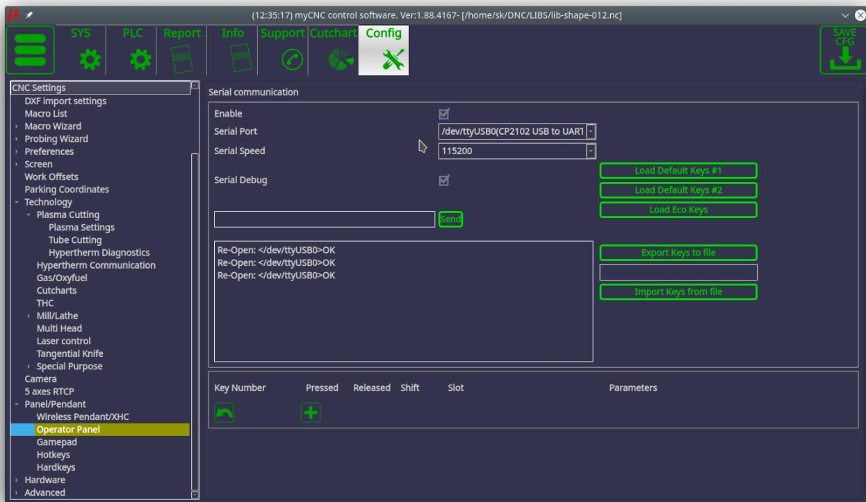
2) To establish communication, you must set the check marks for *Hypertherm Serial Interface* and *Host PC to Hypertherm Interface* to ON:
