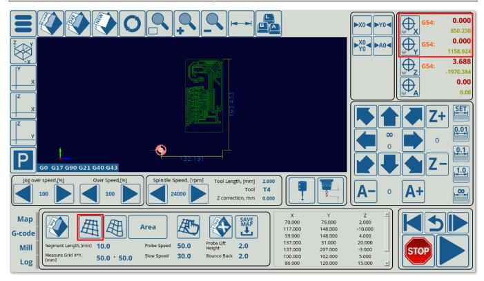
• Press the Run button (this begins the probing process)
