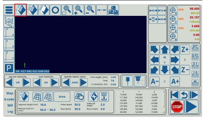
• After opening the file, head to the Map tab on the main screen of myCNC software
