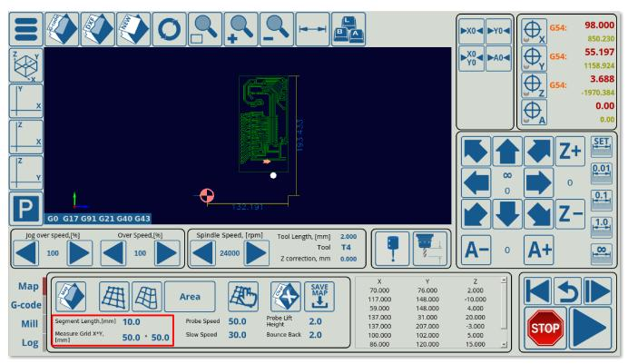
• Select your probe speeds. The probe speed is the speed with which the probe will be moving down from the start of the downward movement to the first contact with the surface. The slow speed is the speed on the rebound, allowing for a more precise measurement of the z-height position on second contact.
