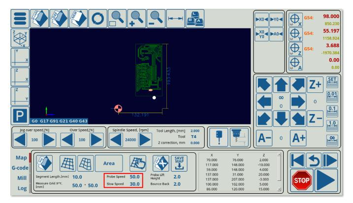
• Select your Lift Height and Bounce Back settings. The Lift Height specifies the z-axis height to which the probe will be lifted between different probing points (safe height). Note that this height is absolute, not relative, so it will raise it TO the position specified in this field in program coordinates, NOT raise the probe BY that amount. The Bounce Back setting specifies the distance the probe retracts after first coming into contact with the working material surface
