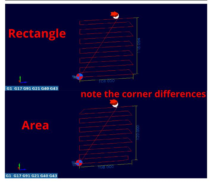
• Press the Generate Map button. Note that in order for the map to position itself properly, the X and Y program coordinates must be at zero prior to the map generation step.
