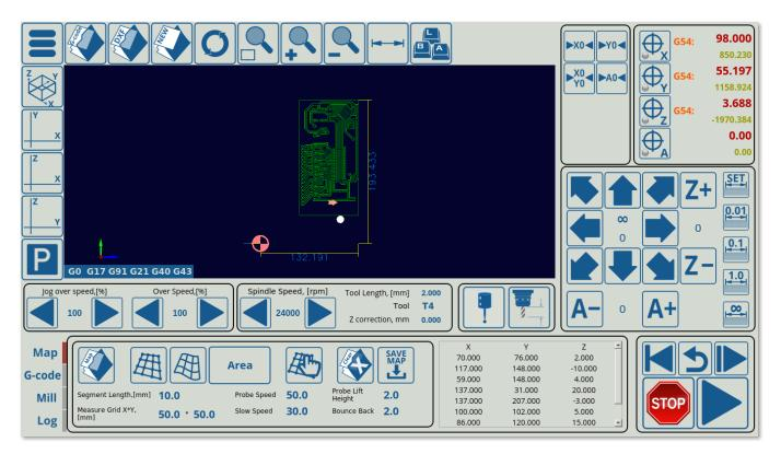
• Select your Segment Length and your XY Grid. Increasing segment length and XY grid will result in less probe points being taken.
