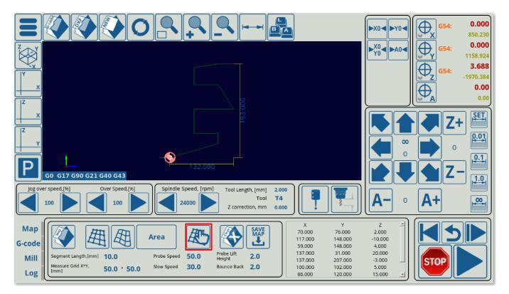
• If you would like to clear the existing generated map (for example, for the purposes of manually recording a set of points without data from the automatic measurements), you can do so using the Clear Map button.
