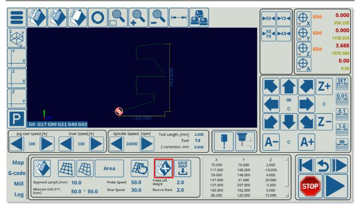
If you would like to save the existing map in order to apply it to a G-code file at a later point, you can do so using the Save Map button. The map will be saved in the folder specified in Settings > Config > Technology > Special Purpose > Height Map.
