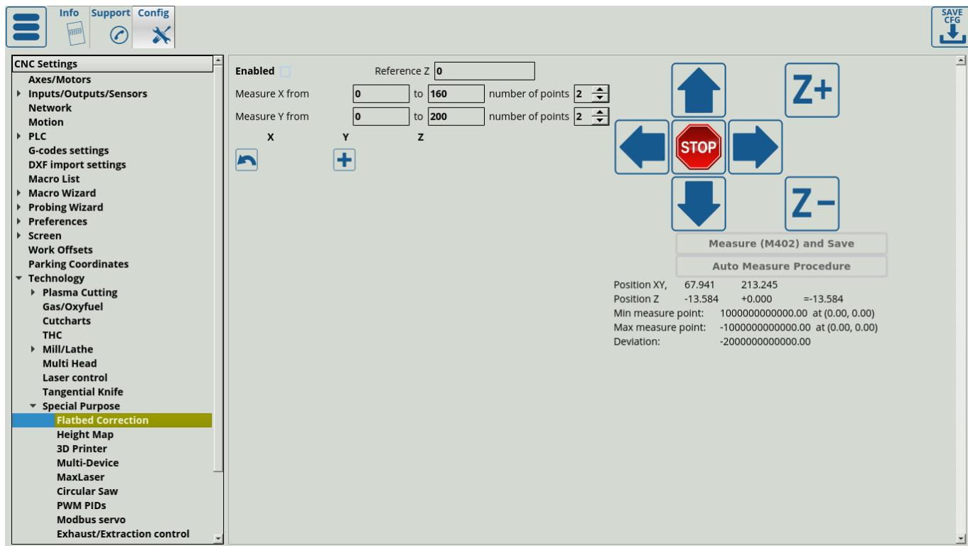
After the setup process has been completed, a table of points in the XY-plane and their Z-positions will be presented on this page. These values can either be recorded by using the AutoMeasure procedure, or by using a sensor and recording each point individually by using the M402 macro. Using the AutoMeasure procedure, the operator can set the measurement distances for the X and Y axes as well as the number of points at which the height measurements will be taken for the XY-plane.
