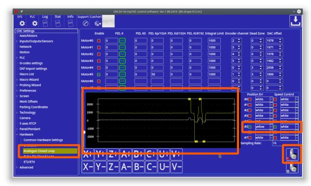
Check which Axis the PID controller attached to (Y axis for the screenshot below).
