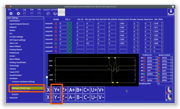
An analogue servo driver normally has a linear function of rotation speed depends on input voltage. A linear coefficient of this function depends on Servo driver and motor, gears, ballscrew etc.
