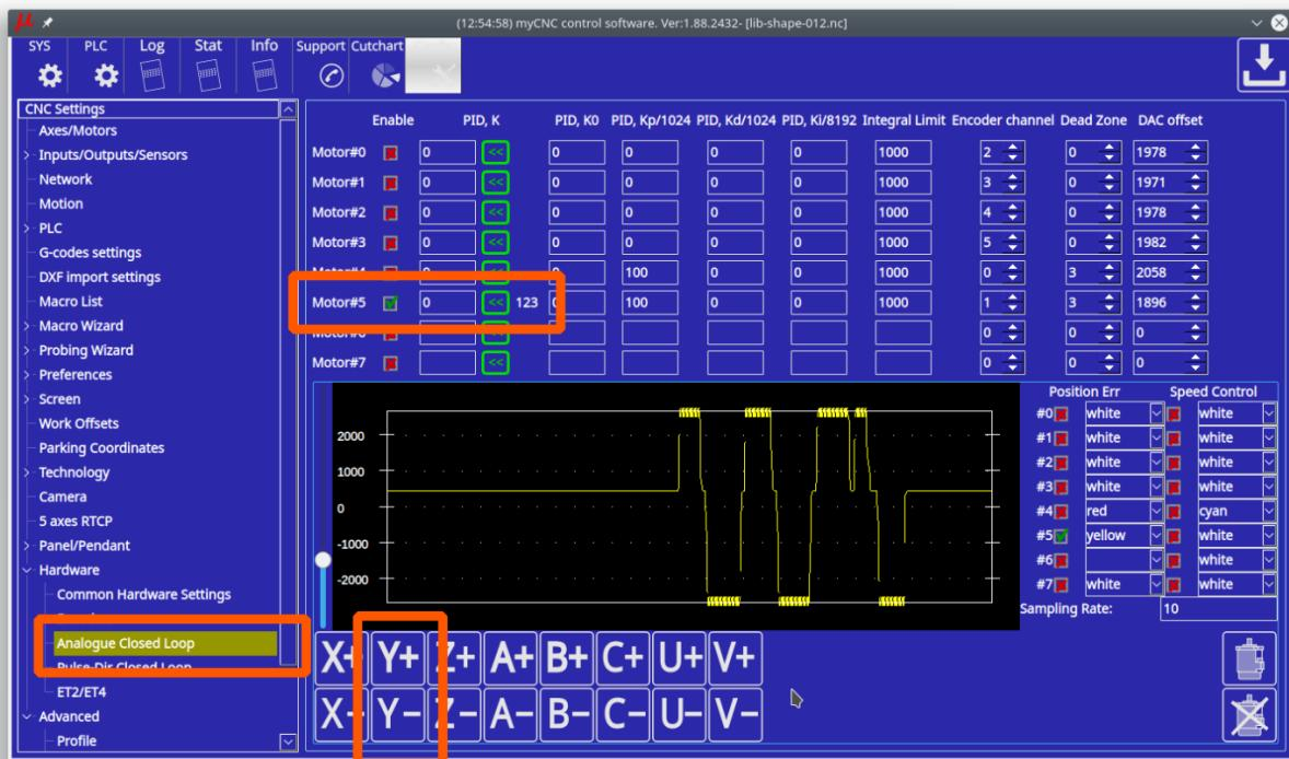
The value can be tuned manually. If rotate a motor shaft with speed more than 20 turns/sec, the controller calculates real Speed/Voltage coefficient and print it on the configuration widget. You can use this value as information to tune the PID **K** ratio. A button  $\leftarrow$  to the right of **PID K** input line can be used to copy the measured **K** ratio to **PID K**.
