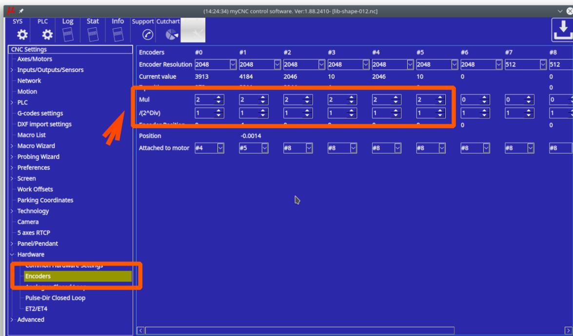
Multiplicator and divider ratio needed for pulse-dir closed loop system to adjust encoder resolution (encoder lines-per-rotation) to motor driver pulse-dir resolution.
