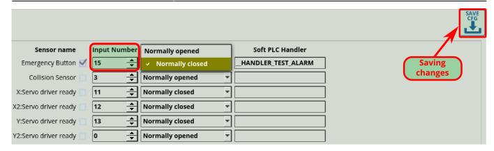
The type of the sensor is specified in the corresponding field "". There are two types of input sensors. Normally open - the sensor in the rest position has open contacts and in the course of operation the sensor contacts are closed. Normally closed - the sensor in the rest position has closed contacts and during the operation, the sensor contacts are opened. This "normal" behaviour can be reversed in Settings > Config > Hardware > Common Hardware Settings > Input Bits Inversion:
