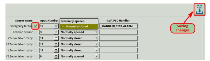
• The input number on the controller board is set in the corresponding field "Inputs Number". Numbering of inputs can be found in the documentation for the selected window controller:
