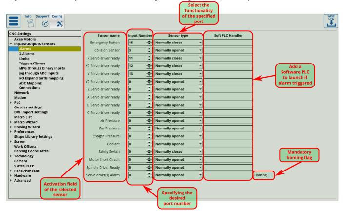
• The selected sensor is activated by setting the "V" symbol in the corresponding field:
