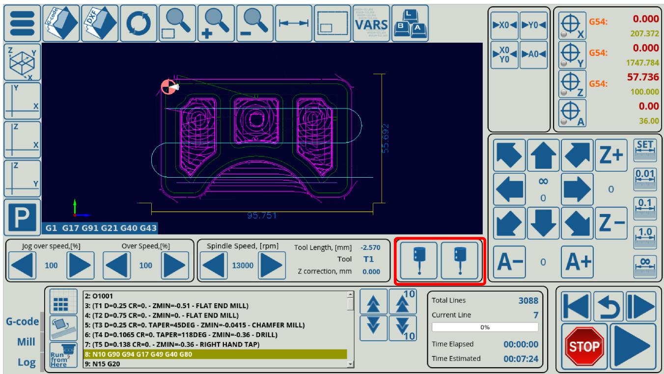
It is also possible to delete the old centring button entirely, to edit it so as to use it as a tool measure button, or to assign a completely different display element in its place (as two probe buttons are unnecessary).
