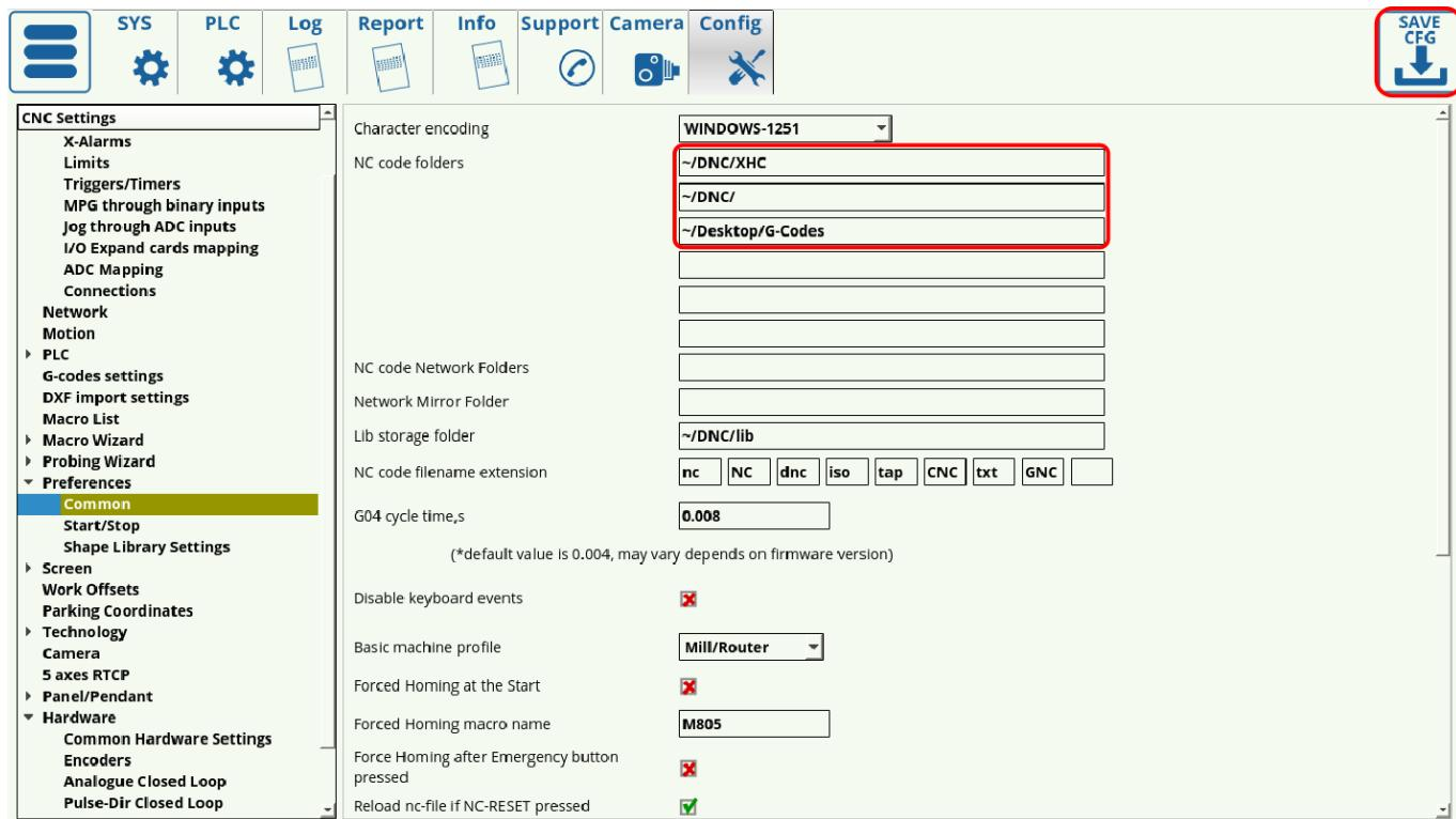
The screenshot shows the 'Config' tab in the myCNC software. On the left, a sidebar lists various settings categories. The 'Common' category is selected and highlighted in yellow. The 'NC code folders' section is highlighted with a red box, showing paths like ~/DNC/XHC, ~/DNC/, and ~/Desktop/G-Codes. A 'SAVE CFG' button is in the top right corner.
